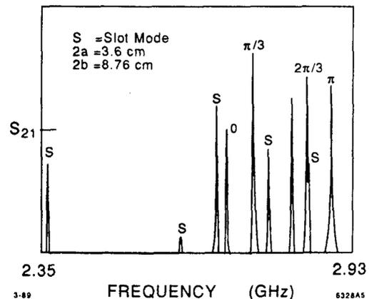
Fig. 5.  $S_{21}$  Plot: Small beam aperture, slots aligned.
