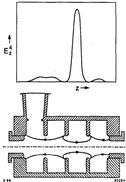
Fig. 7. Cross-section of high-power test structure, with axial field profile.
