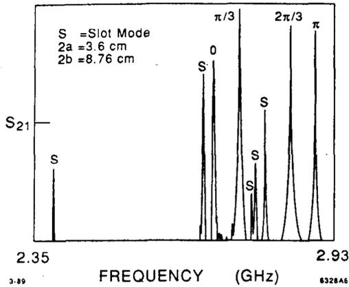
Fig. 6.  $S_{21}$  Plot: Small beam aperture, slots at  $45^\circ$ .
