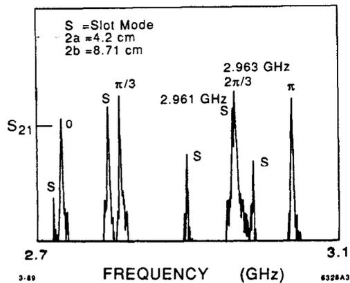
Fig. 3.  $S_{21}$  Plot: Large beam aperture, slots aligned.
