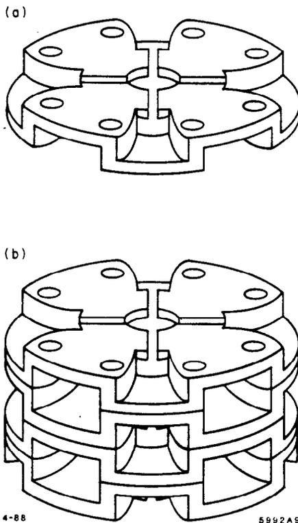
Fig. 1. Accelerator structure with  $HEM_{11}$ -mode damping.
