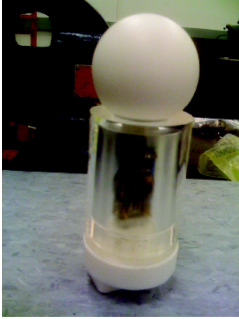
Figure 3.19: Prototype of LED flasher. The diameter of the diffuser ball is 2 inches [183].
