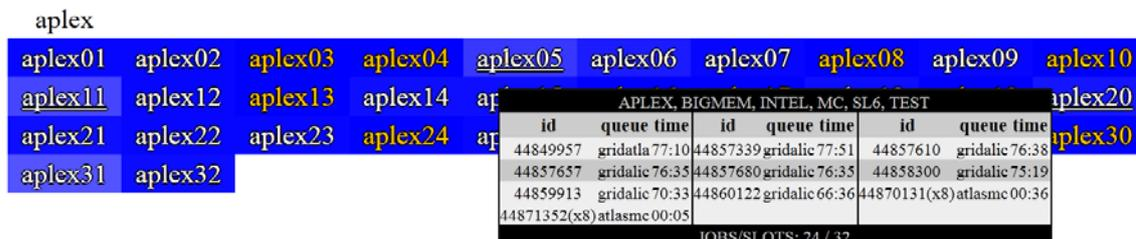
Figure 4: An example of a local monitoring of worker nodes' usage. The source information is parsed from the Torque server. Different colors denote different states of worker nodes. A mouse hover action displays details about running jobs on a selected node.
