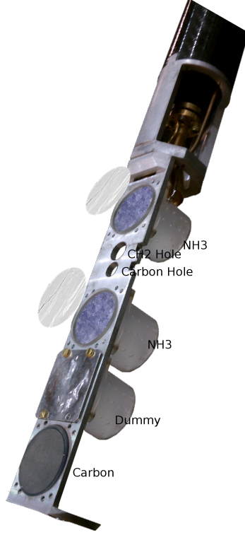
FIGURE 5.7: Target setup on the target stick for the g2p experiment.
