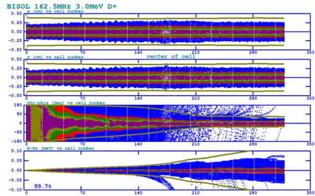
Figure 4: Beam transmission along the RFQ. (Plots from top to bottom are the beam profiles in x and y planes, phase and energy spectrums respectively).
