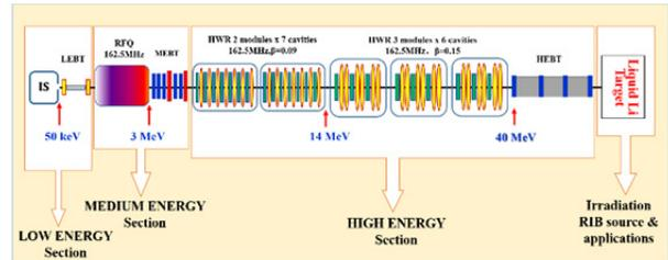
Figure 2: Layout of the high-intensity driver accelerator.
