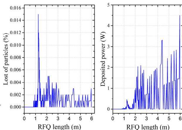
Figure 7: Lost particles (left) and deposited power (right) along the RFQ.
