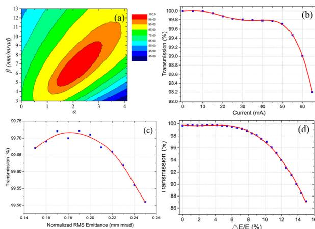
Figure 8: Transmission efficiency of the RFQ behavior versus (a) beam Twiss parameters; (b) beam current; (c) beam emittance and (d) beam energy spread.
