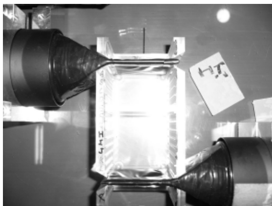
Figure 2. The target box of \text{SiO}_2 set between the plastic scintillation counters
