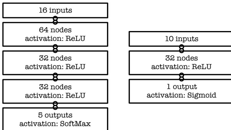
**Figure 4.** Two neural network architectures for jet substructure classification. (Left) A three-hidden-layer model we use to categorize five classes of jets ( $q$ ,  $g$ ,  $W$ ,  $Z$ , and  $t$ ). (Right) A one-hidden-layer model used to identify top quarks, simplified for the FPGA implementation described in section 3.3.
