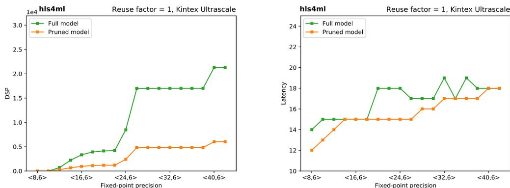
**Figure 11.** A comparison between the compressed and uncompressed models, with a reuse factor of 1 for DSP usage (left) and latency in clock cycles for a 200 MHz clock frequency (right). The x-axis is a scan in the fixed-point precision of the model and demonstrates how resource usage changes as a function of the precision of the calculations in the network inference.
