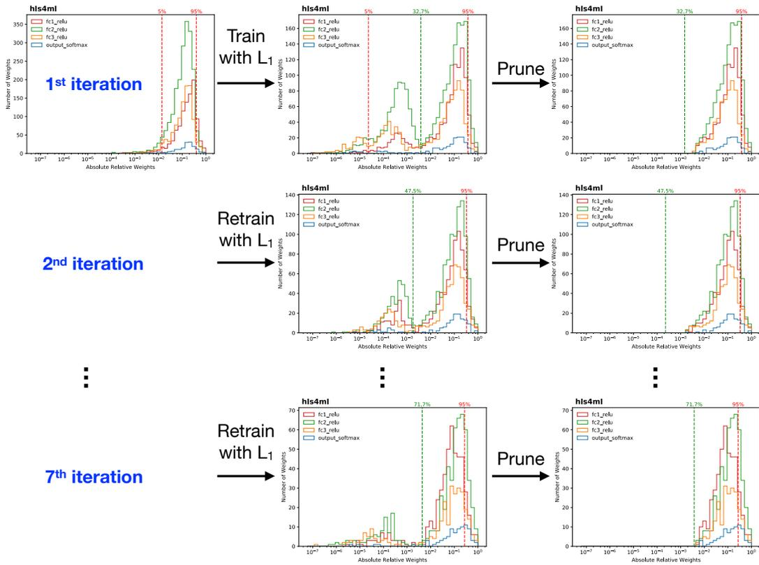
**Figure 6.** Illustration of the iterative parameter pruning and retraining with  $L_1$  regularization procedure. The distribution of the absolute value of the weights relative to the maximum absolute value of the weights is shown after each step of the pruning and retraining procedure. In the top left, the distribution before compression is shown, while in the bottom right, the distribution after compression is displayed.
