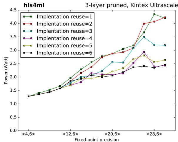
**Figure 15.** Power usage (W) for the baseline three-hidden-layer model as a function of precision.
