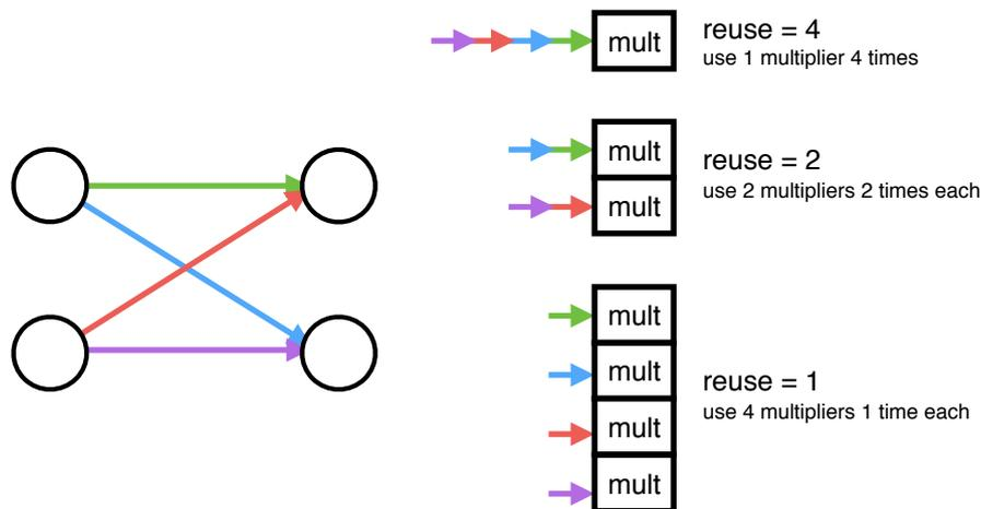
**Figure 8.** Illustration of multiplier resource usage for different values of reuse factor. The left drawing shows the case of two neuron pairs being connected by 4 connections, implying four multiplications to be performed. The right drawing shows how to perform these multiplications, from fully serial (top) to fully parallelized (bottom).
