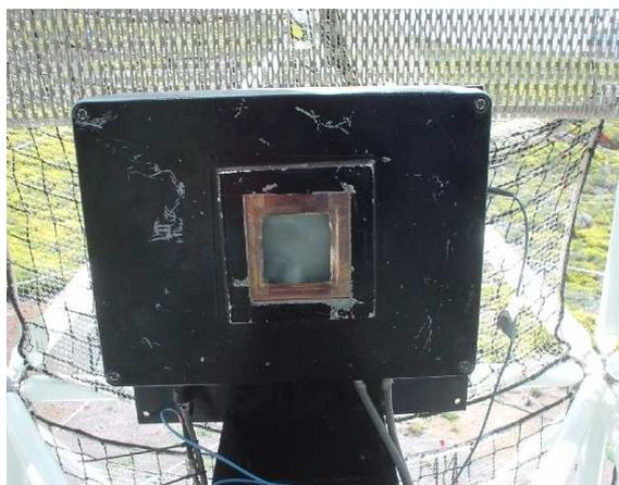
Figure 6.11: Calibration pulser box installed in the middle of the telescope mirror dish.
