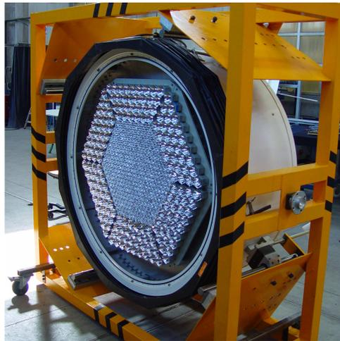
Figure 5.17: The MAGIC camera ready to be shipped from IFAE to La Palma with the light collectors matrix already installed.
