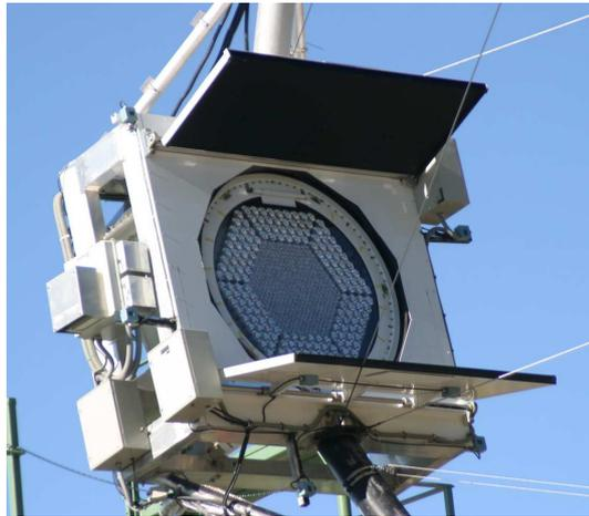
Figure 5.18: Photograph of the MAGIC camera installed in the Telescope frame.
