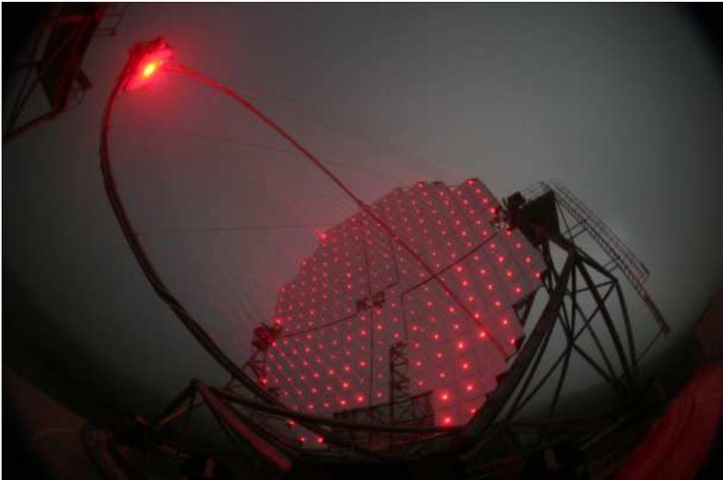
Figure 5.15: Mirror panel lasers switched on during re-alignment procedure. Not all mirror panels were installed at the time of the photograph.
