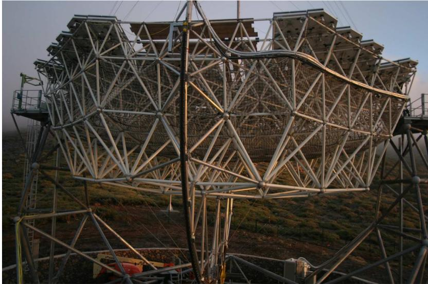
Figure 5.13: MAGIC telescope pointing upwards. In this position, the carbon fiber frame can be photographed easily. Mirrors were partially installed.
