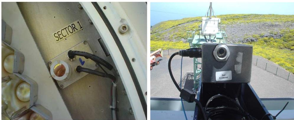
Figure 6.13: Left: One of the three blinded pixels installed in the camera. Right: Pin-diode box installed in front of the pulser box.
