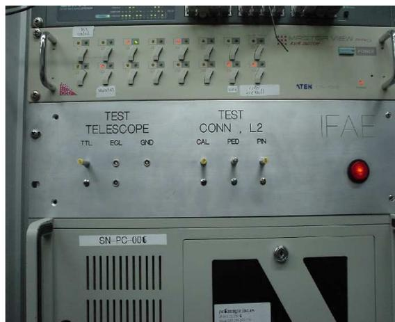
Figure 6.15: Front panel of the calibration trigger board with the test lines and indicator LEDs.
