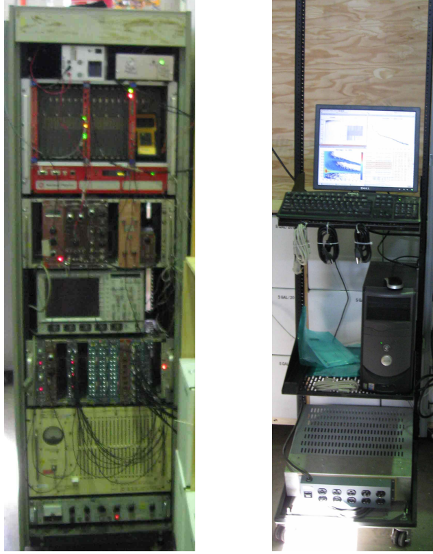
Figure 3.20: The electronics rack and daq system. Left: the red front-panel crate on the top is the CAEN VME 8100 unit housing one CAEN V1720B digitizer board and one crate controller board; the two smaller units on top of VME crates are the DC power supply to the PT1000 sensors and the controller to the liquid argon level maintaining system; the rest are (from top to bottom): high voltage power supply to the inner PMT and (pre-)amplifiers, oscilloscope, logic modules for the veto signal processing, and HV distributor and HV power supply for the veto PMTs. Right: the data acquisition computer showing some online analysis results.
