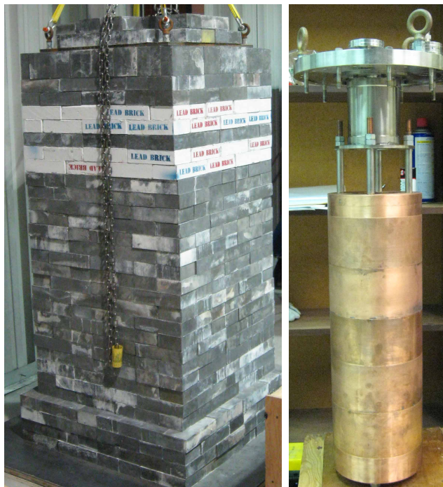
Figure 3.13: Gamma ray shielding of the low background detector. Left: the lead castle; the wall thickness is 8" around the detector sensitive volume, 6" around the flanges and feedthroughs, and 4" to the top. Right: the outer copper shielding that hangs inside the lead castle; another 2.5" thick copper plug closes the top inside the inner detector cylinder.
