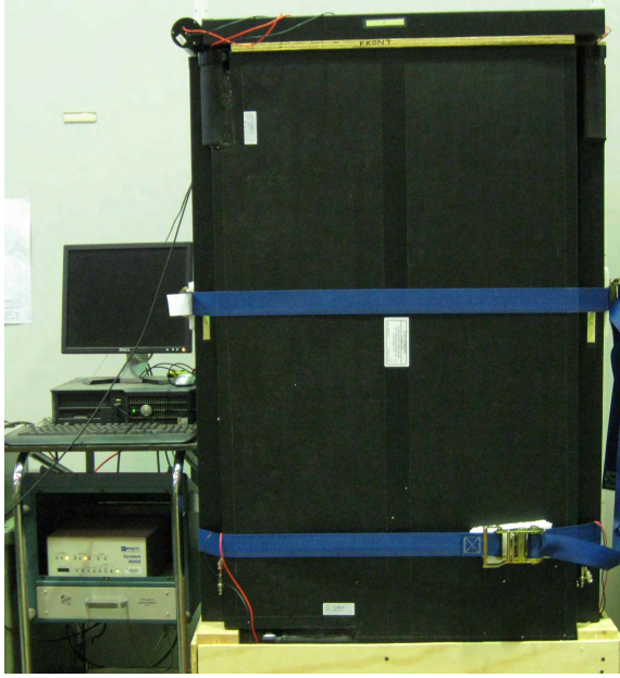
Figure 3.14: The muon veto panels mounted outside the lead shielding.
