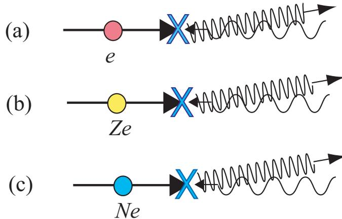
Figure 3: Compton scattering processes of photons from (a) single electron, (b) atomic nucleus with a charge  $Z$ , and (c) a beam bunch with  $N$  electrons. The scattering cross sections are given by  $\sigma_T^e = \frac{8\pi}{3} \left( \frac{e \times e}{4\pi\epsilon_0 mc^2} \right)^2 = 6.7 \times 10^{-25} \text{ cm}^2$ ,  $\sigma_T^Z = Z^2 \sigma_T^e$ , and  $\sigma_T^N = N^2 \sigma_T^e$ , respectively.
