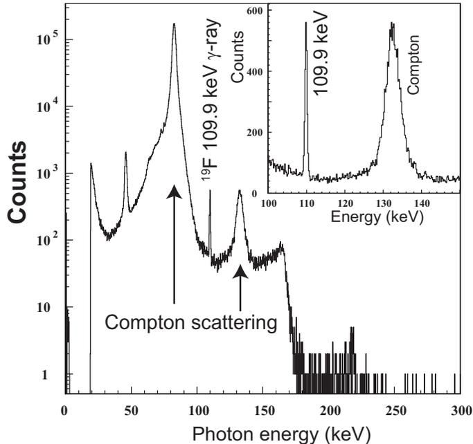
Figure 7: Photon spectrum to demonstrate the nuclear resonance fluorescence  $\gamma$ -rays from the 109.9 keV level in  $^{19}\text{F}$ . A 110 keV Wiggler photon beam with an energy resolution of about 100 eV has been used at SPring-8.
