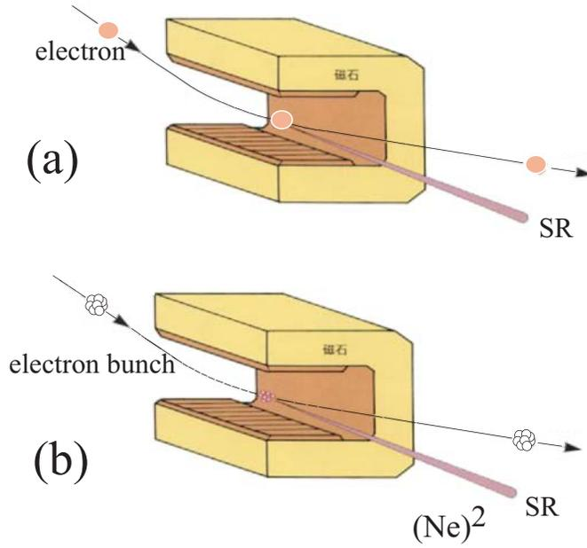
Figure 2: Synchrotron radiation with a single electron and an electron bunch with a number of  $N$ . If the  $N$  electrons in the bunch are bent in coherent in a dipole magnet, the synchrotron radiation from the electron bunch is enhanced by a factor of  $N^2$  compared with that from a single electron.
