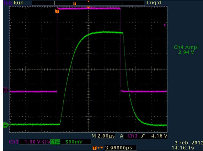
FIG. 7: Example of pulse shape shown on an oscilloscope for pervance measurement: modulator voltage (purple trace) and collector current (green trace).
