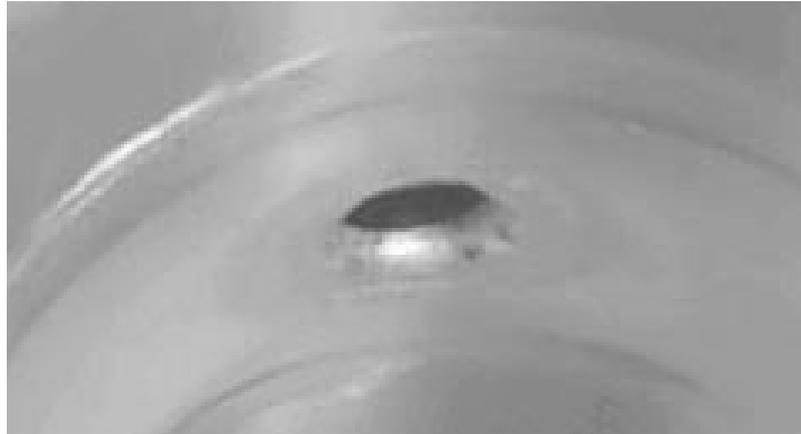
Figure 4.11: A picture of the high-power coupling aperture of cavity 1 after the first high-power test. Near the aperture, the magnetic field is in the up-down direction and the electric field is in the left-right direction. The aperture has been rounded in the up-down direction, and pitting has occurred to the left and the right of the aperture.
