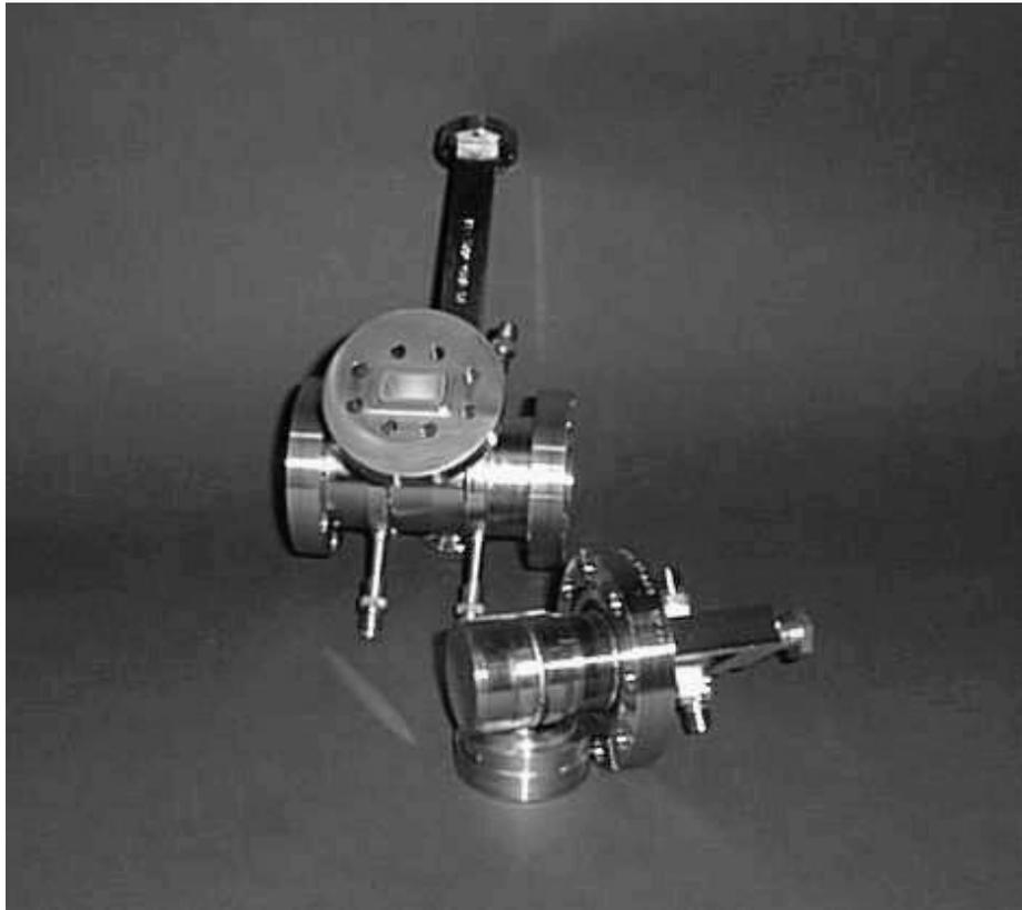
Figure 2.26: Cavity body with endcap shown on the outside. The water-cooling pipes can be seen on the bottom of the cavity body.
