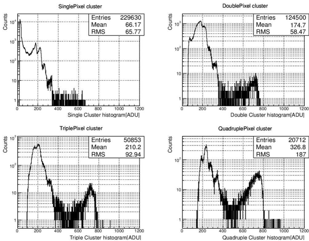
FIGURE 4.19: Distributions of amplitudes generated in DIPIX2 FZ-p by Am-241 X-ray source for different cluster size.
