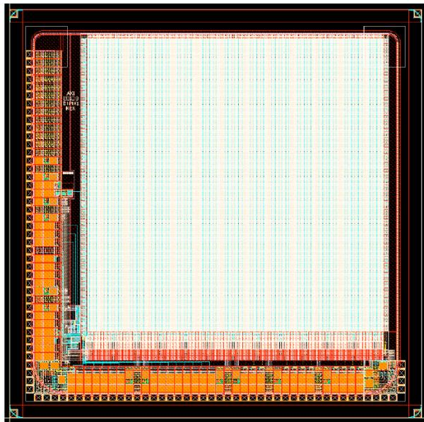
FIGURE 4.3: Chip layout of DIPIX2.
