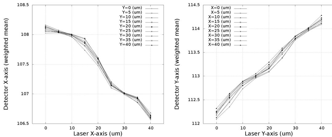
FIGURE 3.19: The weighted mean of the cluster of hit pixel (with laser) is calculated with respect to laser position. The laser is moved by  $40 \times 40 \mu\text{m}$  with a step of  $5 \mu\text{m}$ .
