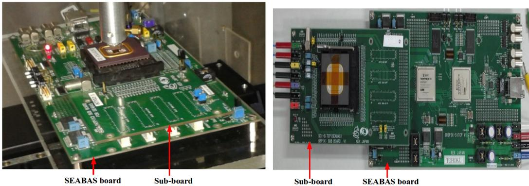
FIGURE 4.29: INTPIX3 (left) and DIPIX2 (right) seabas and sub-board.
