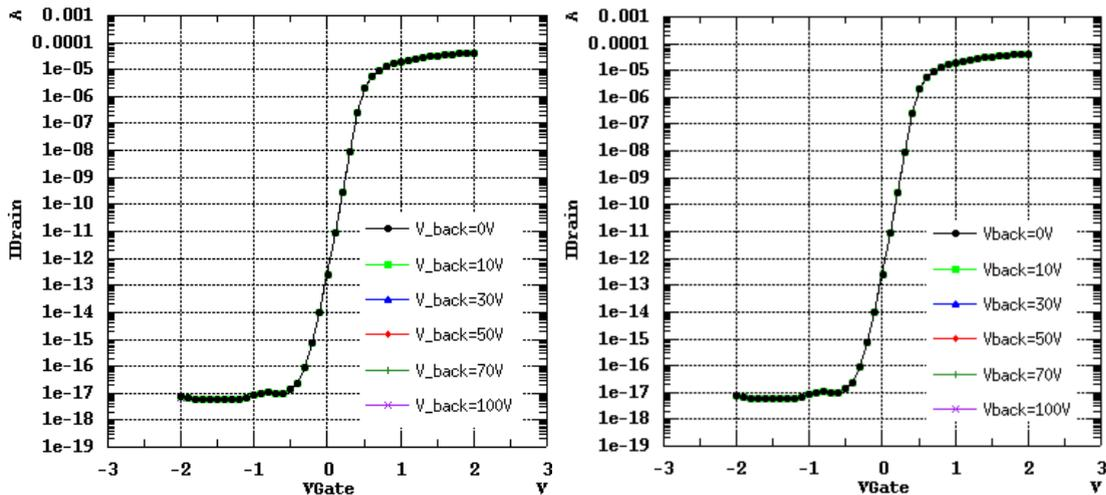
FIGURE 2.3: Transfer characteristic of NMOS IO transistor at different sensor back bias voltages. The transistor is placed at the top of the pixel and back gate effect is studied by varying the BPW size from  $1 \mu\text{m}$  (left) to  $8 \mu\text{m}$  (right).
