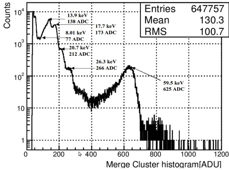
FIGURE 4.18: Energy spectra of X-ray (Am-241) obtained after merging all clusters from DIPIX2 CZ-n.
