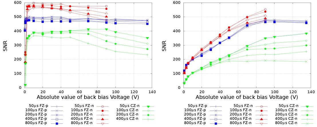
FIGURE 4.14: Signal to noise ratio as a function of detector bias voltage obtained at different integration times with 660 nm laser (left) and 1060 nm laser (right) for DIPIX2 CZ-n, FZ-n and FZ-p.
