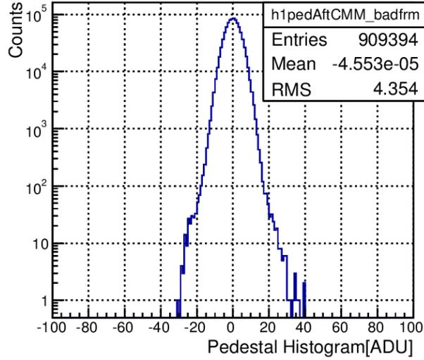
FIGURE 3.21: Histogram of the Pedestal after common mode rejection and masking bad pixel (6<sup>th</sup> region of INTPIX3a).
