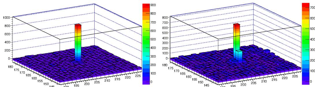
FIGURE 4.11: Examples of laser events of DIPIX2 CZ-n detector illuminated with 660 nm (left) and 1060 nm (right) laser wavelength.
