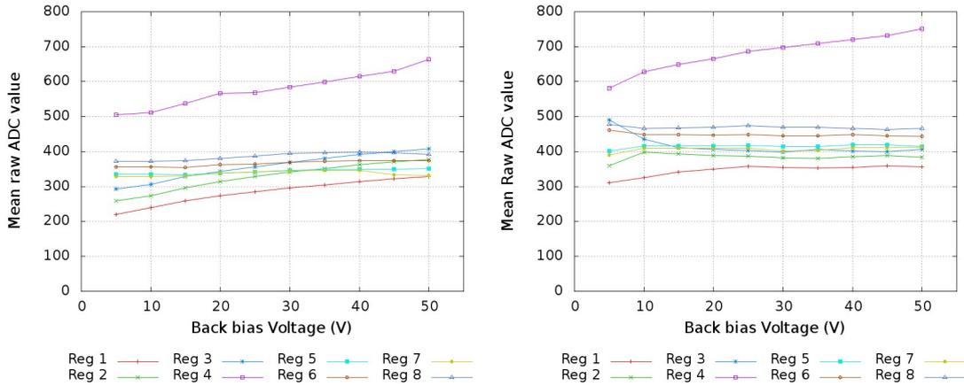
FIGURE 3.16: Mean raw pixel output (in ADC counts) as a function of detector bias voltage of INTPIX3a, floating (left) and constant (right) guard voltage (Pedestal Shift).
