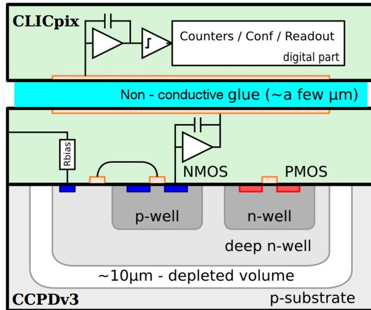
FIGURE 1.13: Schematic view of one pixel cell of a CCD. After [64].
