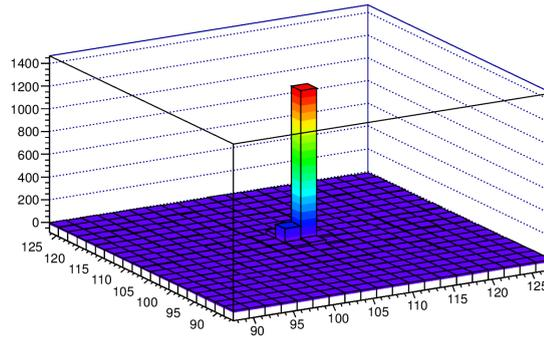
FIGURE 3.18: 2-D laser histogram of single pixel for 8<sup>th</sup> region of INTPIX3a.
