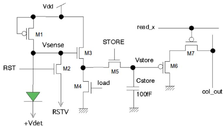
FIGURE 3.12: Single pixel circuit of INTPIX3.
