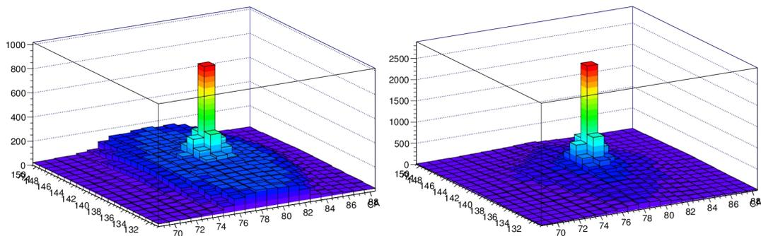
FIGURE 4.8: 2-D plot of DIPIX2 FZ-n detector before (left) and after (right) optimisation of the laser spot.
