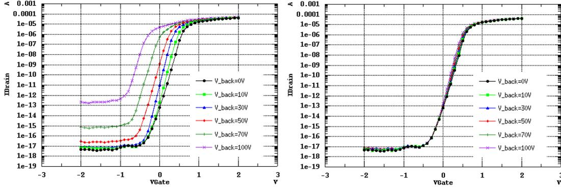
FIGURE 2.4: Transfer characteristic of NMOS IO transistor at different sensor back bias voltage. The transistor is placed between two pixel and back gate effect is studied by varying the BPW size from  $1 \mu\text{m}$  (left) to  $8 \mu\text{m}$  (right).
