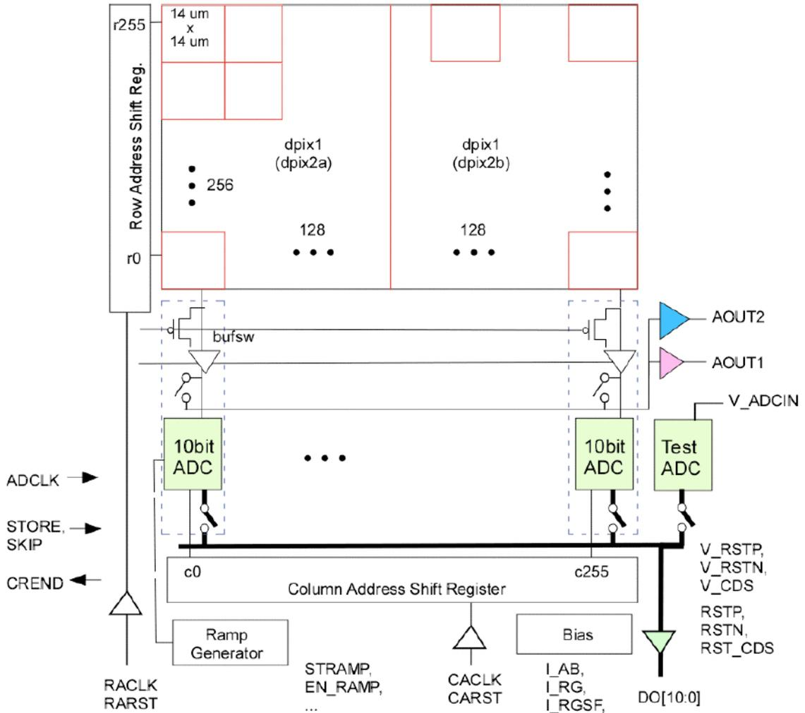
FIGURE 4.1: DIPIX2 block diagram.
