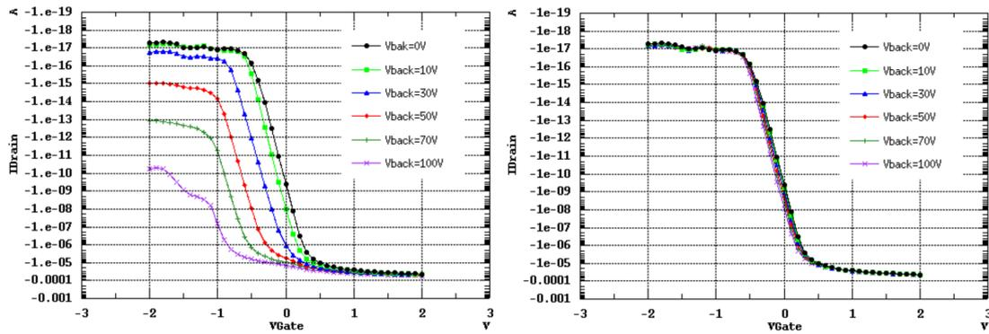
FIGURE 2.5: Transfer characteristic of PMOS IO transistor at different sensor back bias voltage. The transistor is placed between two pixel and back gate effect is studied by varying the BPW size from  $1 \mu\text{m}$  (left) to  $8 \mu\text{m}$  (right).
