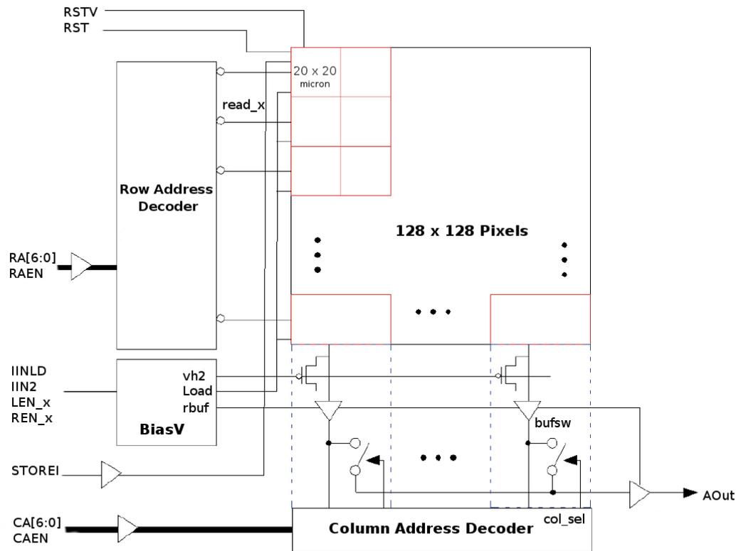
FIGURE 3.11: INTPIX3 block diagram.
