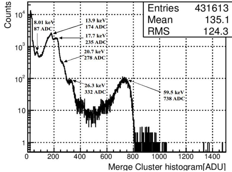
FIGURE 4.20: Energy spectra of X-ray (Am-241) obtained after merging all clusters from DIPIX2 FZ-p.
