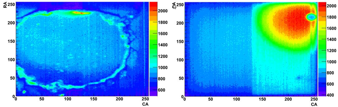
FIGURE 4.6: 2-D plot of DIPIX2 FZ-n detector represents ADC counts as a function of pixel matrix. Halo effect at high detector bias voltage (left: 100 V) and a cluster of hot pixels at low detector bias voltage (right: 0V).
