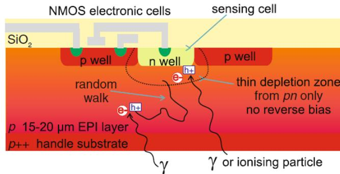
FIGURE 1.9: Schematic view of one pixel cell of a MAPS. After [38].
