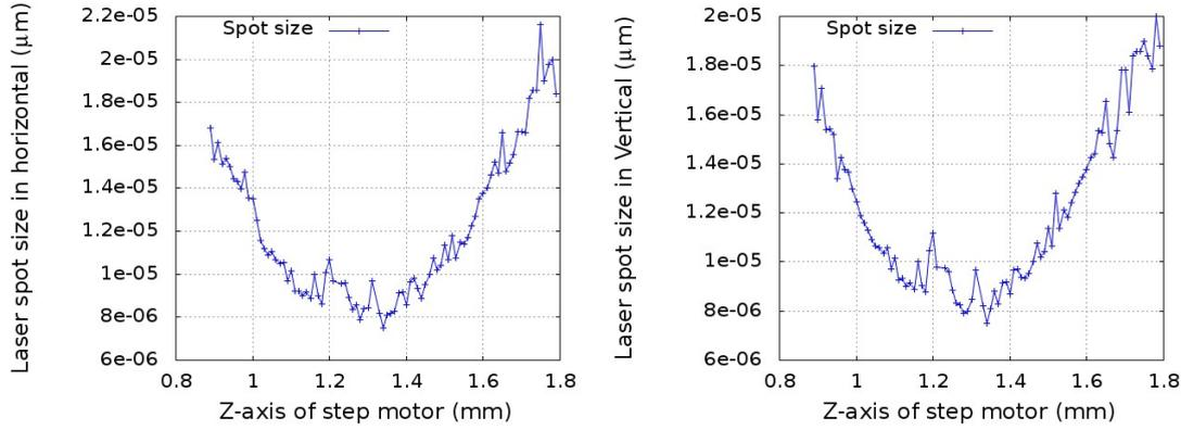
FIGURE 3.17: Spot size of hit pixel (with 660 nm laser) is calculated in Horizontal (left) and Vertical (right) direction with respect to distance between laser and detector for 8<sup>th</sup> region of INTPIX3a.
