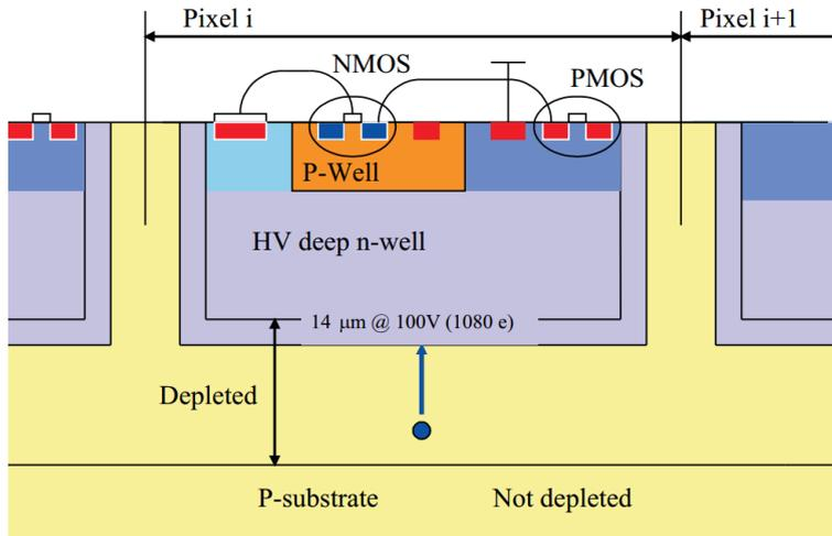
FIGURE 1.12: Schematic view of one pixel cell of a HV-CMOS. After [62].
