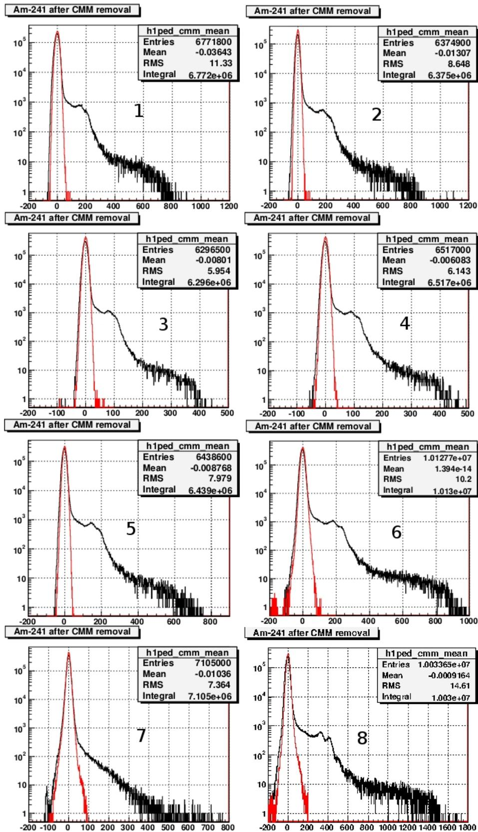
FIGURE 3.26: Histogram of all region in INTPIX3b. The pedestals are represented in red and the signal from Am-241 is represented in (black). (The numbers in the figure indicate the region number of INTPIX3b).
