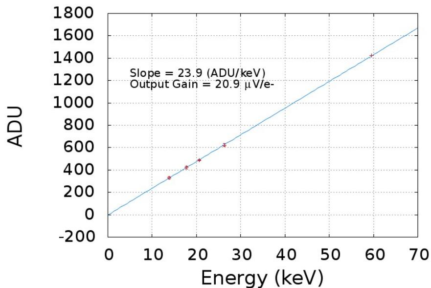
FIGURE 3.30: Output gain of 8<sup>th</sup> region of INTPIX3b calculated using the linear fit of Am-241 spectrum.
