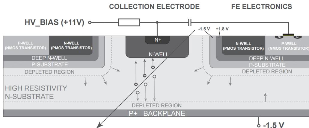
FIGURE 1.11: Schematic view of one pixel cell of a DMAPS. After [60].
