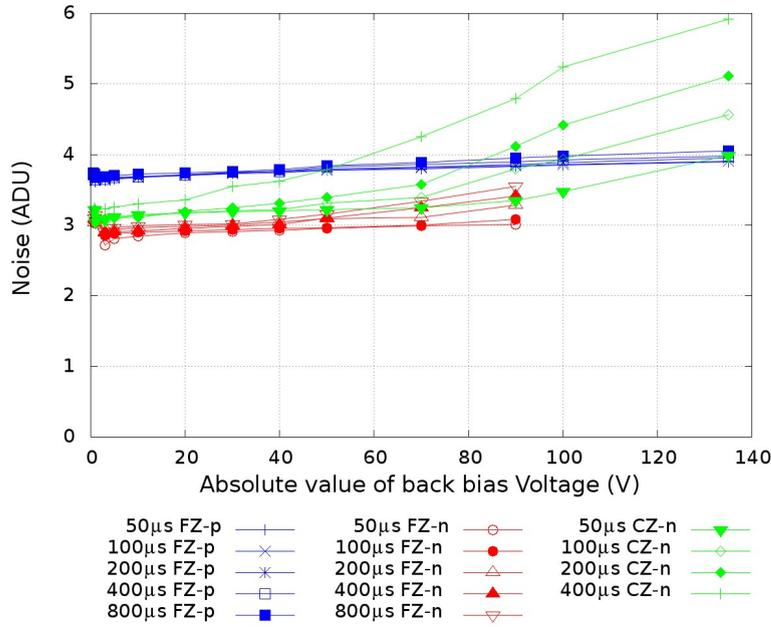
FIGURE 4.13: Noise as a function of detector bias voltage obtained at different integration times with DIPIX2 CZ-n, FZ-n and FZ-p.
