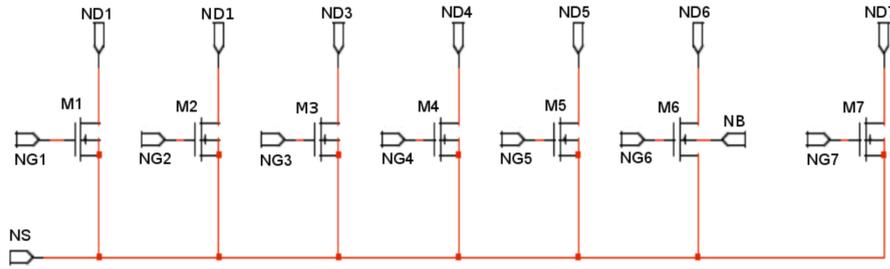
FIGURE 3.8: Circuit diagram of NMOS test transistor.
