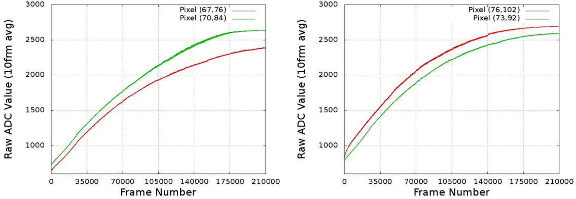
FIGURE 3.15: Raw pixel output (in ADC counts) as a function of time (frame number) for 6<sup>th</sup> region of detector INTPIX3a (left) and INTPIX3b (right).
