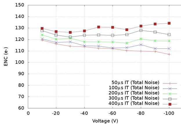
FIGURE 4.28: The ENC noise as a function of the sensor bias voltage for FZ-p detector.
