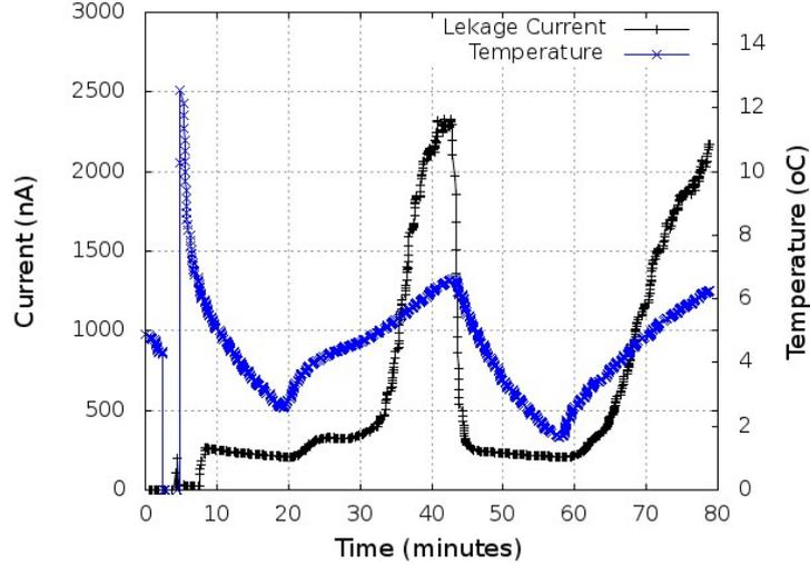
FIGURE 4.15: The FZ-p detector is used to study the dependence of leakage current on temperature with time.
