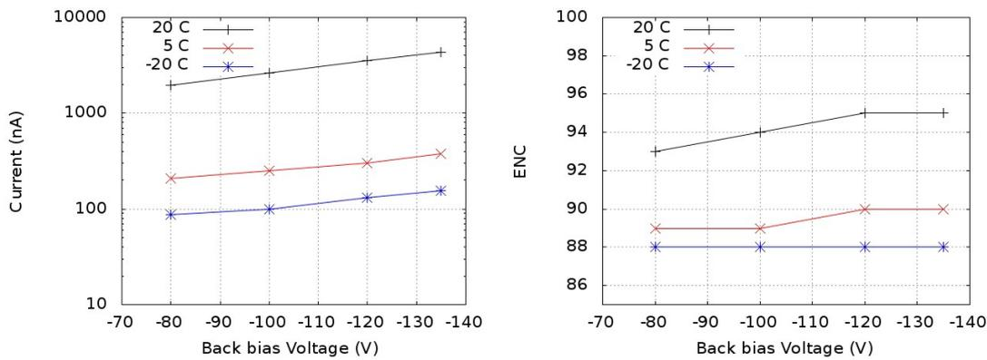
FIGURE 4.23: The FZ-p detector is measured to plot the leakage current (left) and ENC (right) as a function of detector bias voltage at three different temperatures.
