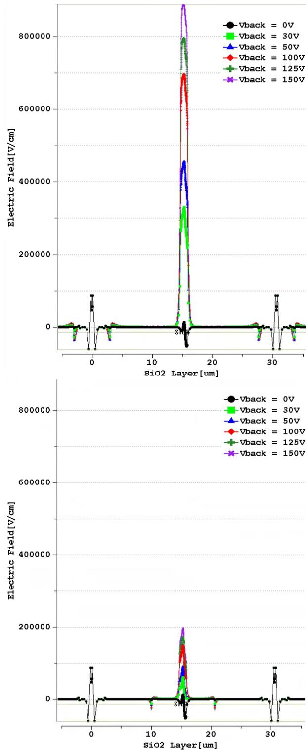
FIGURE 2.7: The back gate effect on transistor is studied by varying BPW size. The electric field distribution of SOI pixel sensor in the oxide layer is shown for two BPW sizes, 1  $\mu\text{m}$  (top) and 8  $\mu\text{m}$  (bottom).
