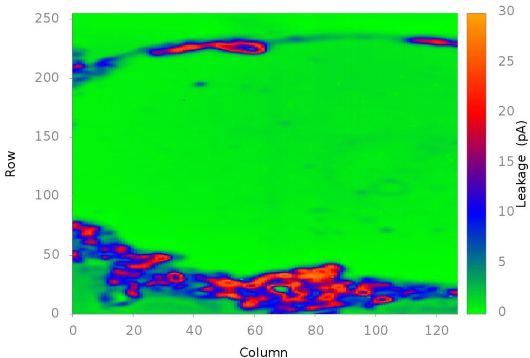
FIGURE 4.7: 2-D plot of 1<sup>st</sup> region of FZ-n detector at 100 V detector bias voltage. Leakage current as a function of pixel position in matrix.
