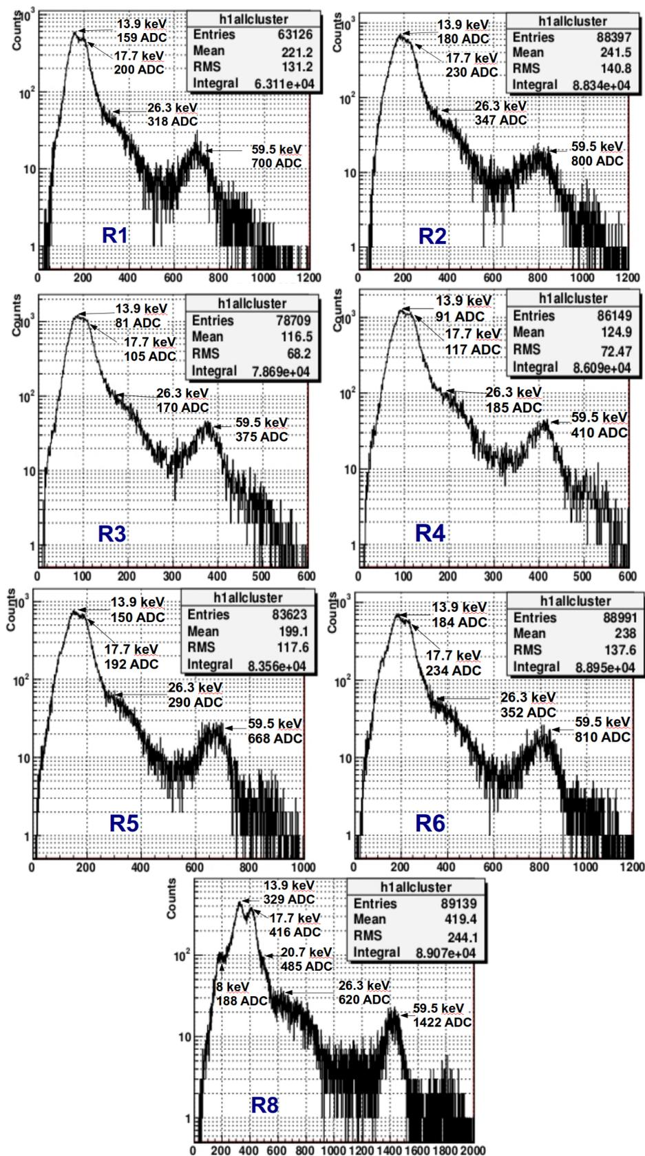
FIGURE 3.28: Histogram after merging all cluster of detector INTPIX3b.
