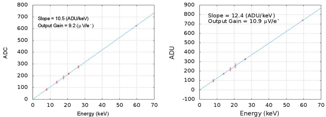
FIGURE 4.21: ADC count as a function of the energy spectrum from Am-241 for CZ-n (left) and FZ-p (right).
