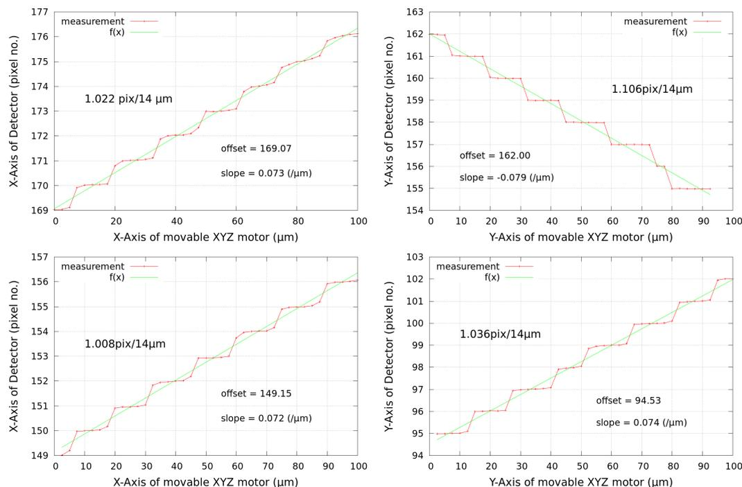
FIGURE 4.10: Pixel scan using 660 nm (top) and 1060 nm (bottom).
