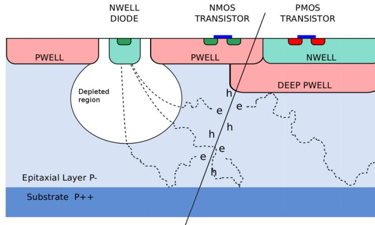
FIGURE 1.10: Schematic view of one pixel cell of a deep p-well with high resistivity partially depleted EPI layer. After [59].
