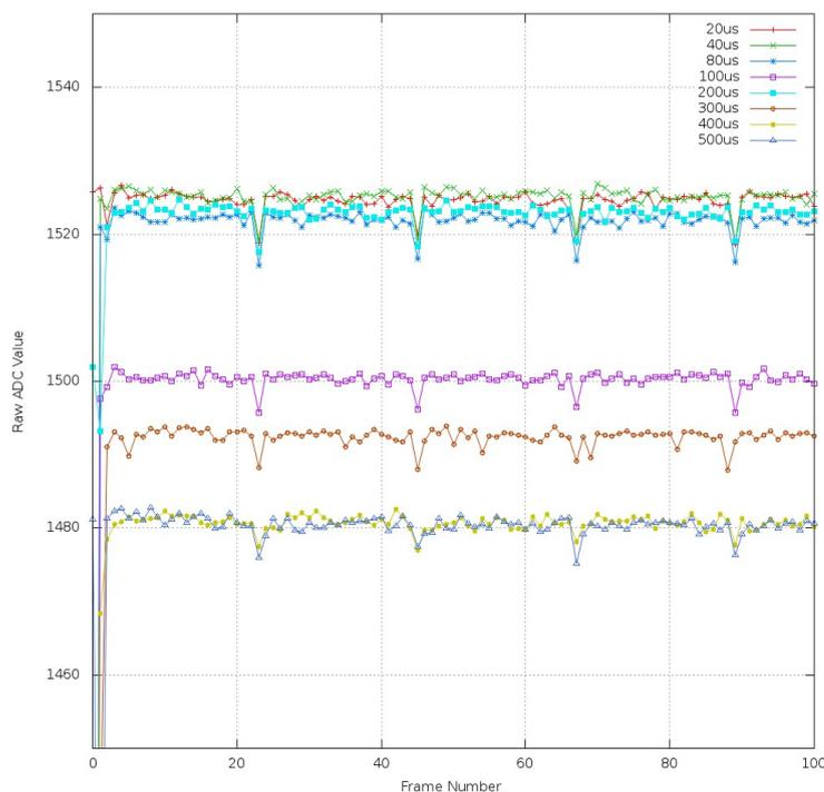
FIGURE 4.9: Periodic noisy peaks in CZ-n detector without CDS. The raw ADC values are a function of frame number for different integration times.
