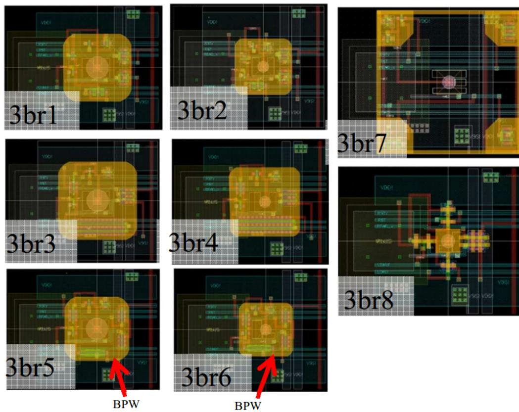
FIGURE 3.14: Pixel layout of INTPIX3b.
