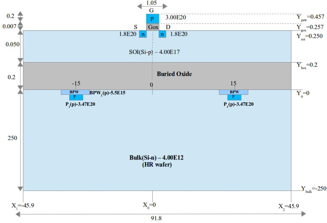
FIGURE 2.2: Geometry of 2-D DIPIX pixel detector prototype with dimensions, material and doping profile details. Note: All dimensions are in  $\mu\text{m}$  and not to scale.
