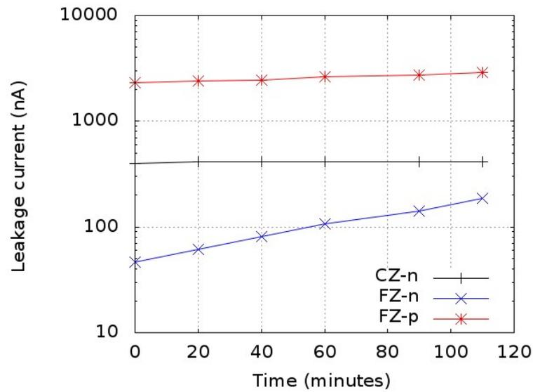
FIGURE 4.16: Leakage current at room temperature as a function of time.
