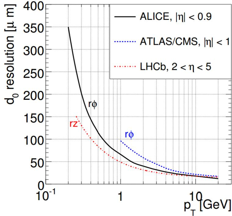
FIGURE 1.3: Track impact parameter resolution for the four LHC experiments. After [29].
