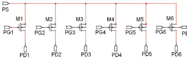
FIGURE 3.9: Circuit diagram of PMOS test transistor.
