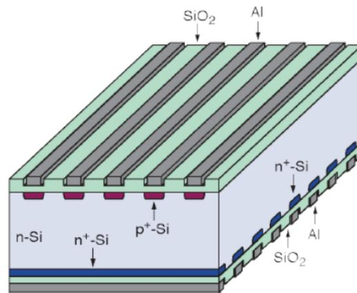
FIGURE 1.7: Schematics showing a double-sided silicon strip detector. After [42]
