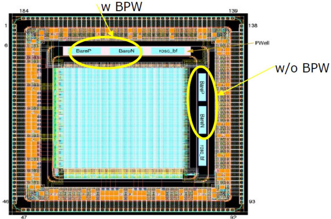
FIGURE 3.7: INTPIX3a layout with transistor location.
