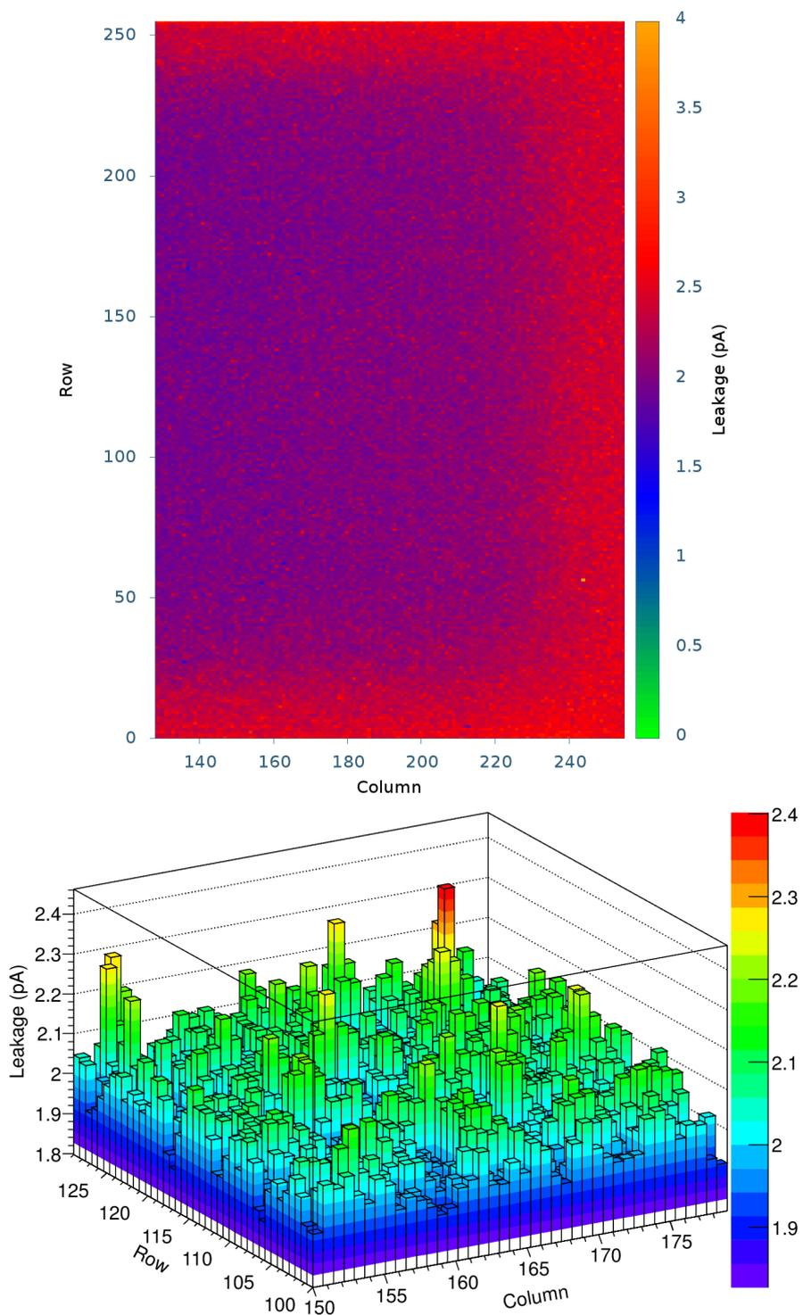
FIGURE 4.25: The pixel currents of the DIPIX2 FZ-p biased to -80 V as a function of the pixel position. Top picture shows currents of 128 x 256 pixel area (half of the sensor) and the bottom one is a zoomed 3D graph of the 30 x 30 pixels area.
