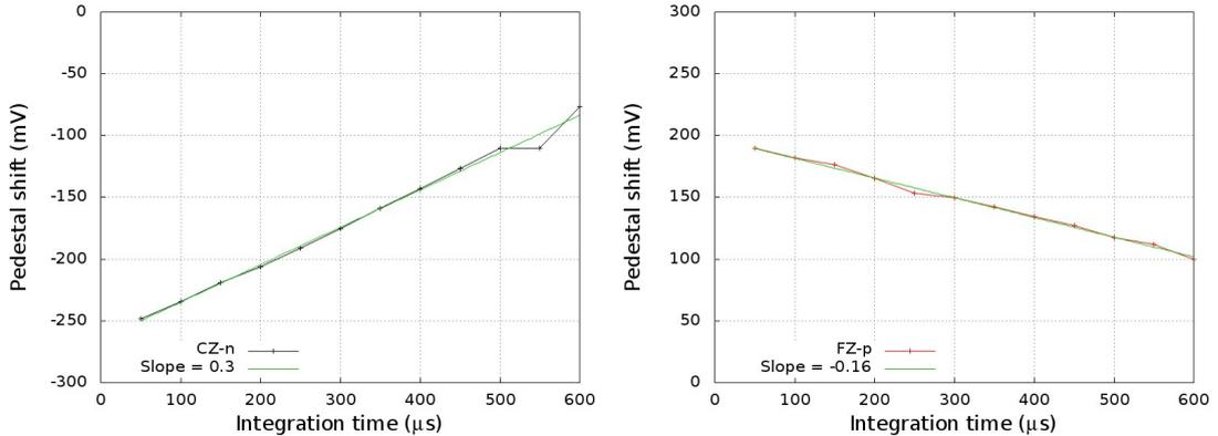
FIGURE 4.24: To calculate the pixel current, mean pedestal shift is plotted as a function of integration time, CZ-n (left) and FZ-p (right).
