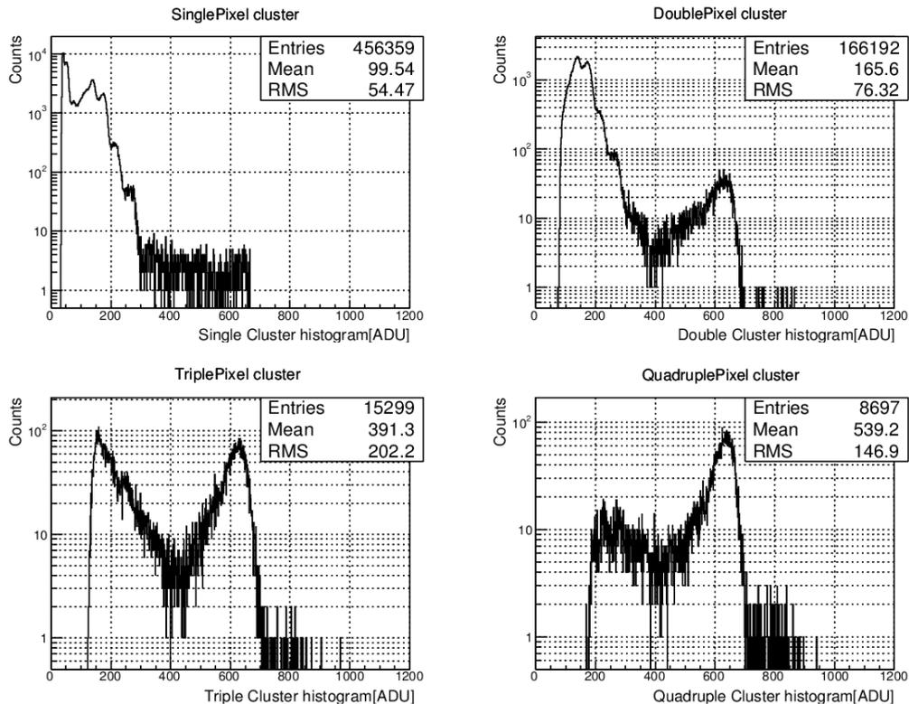
FIGURE 4.17: Distributions of amplitudes generated in DIPIX2 CZ-n by Am-241 X-ray source for different cluster size.
