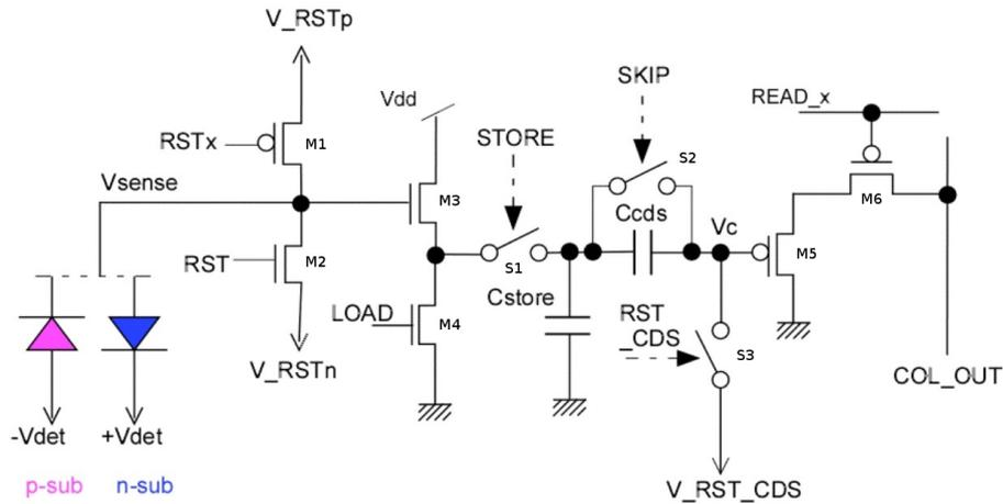
FIGURE 4.2: Single pixel circuit of DIPIX2.
