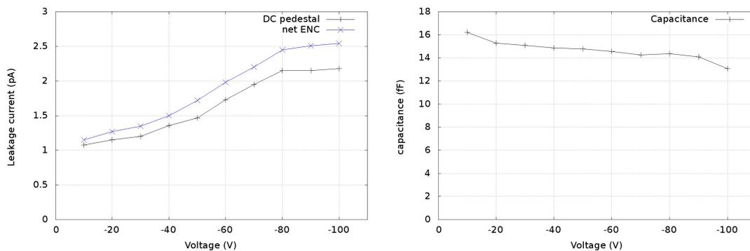
FIGURE 4.27: The FZ-p pixel current (left) and the pixel capacitance vs detector bias voltage.
