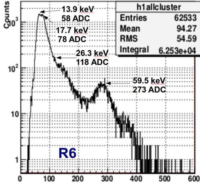
FIGURE 3.23: Histogram after merging all clusters and the peaks indicate the energy of Am-241 in ADC count (6<sup>th</sup> region of INTPIX3a).
