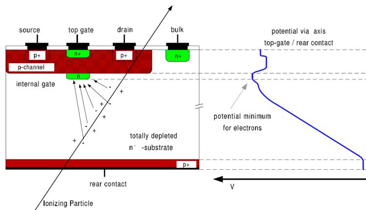
FIGURE 1.14: Schematic view of one pixel cell of a DEPFET. After [67].
