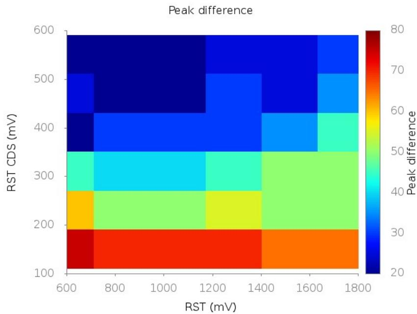
FIGURE 4.26: 2D plot, the peak difference as a function of RST and RST\_CDS.
