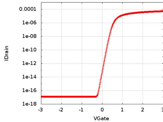
FIGURE 2.6: The transfer characteristic of NMOS IO transistor simulated using Cadence.
