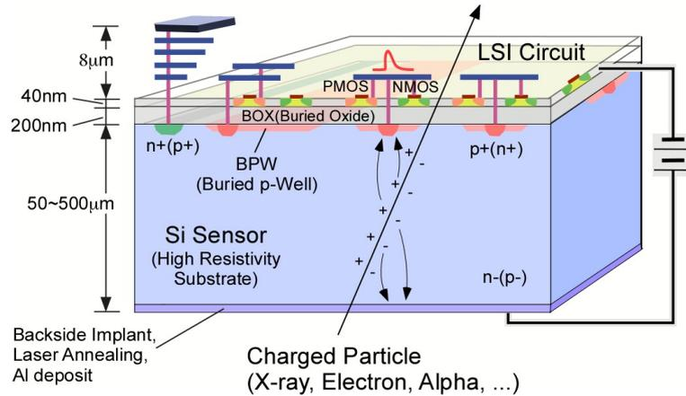
FIGURE 1.15: Schematic view of one pixel cell of a SOI detector. After [73].
