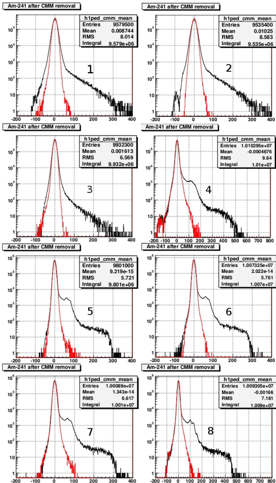
FIGURE 3.25: Histogram of all region in INTPIX3a. The pedestals are represented in red and the signal from Am-241 is represented in (black). (The numbers in the figure indicate the region number of INTPIX3a).
