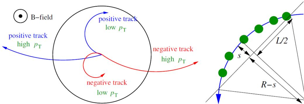
FIGURE 1.1: The deflection of particle track due to a perpendicular magnetic field (left) and its measurement (right). After [25].
