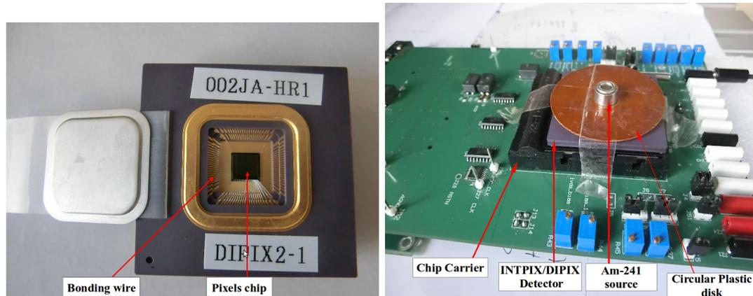
FIGURE 3.1: Radiation source set-up, detector (left) and set-up (right).
