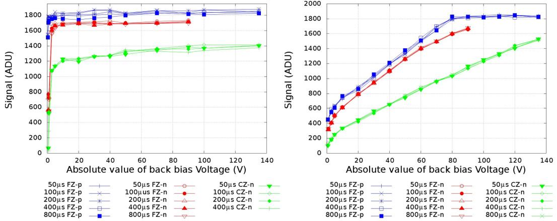
FIGURE 4.12: Signal amplitude as a function of detector bias voltage obtained at different integration times with 660 nm laser (left) and 1060 nm laser (right) for DIPIX2 CZ-n, FZ-n and FZ-p.
