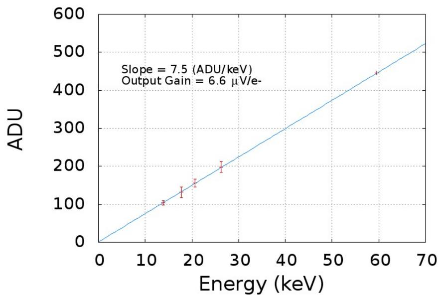
FIGURE 3.29: Output gain of 8<sup>th</sup> region of INTPIX3a calculated using the linear fit of Am-241 spectrum.
