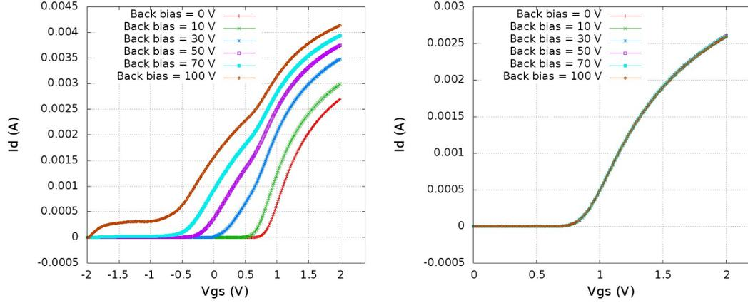
FIGURE 3.10: Transfer characteristic of NMOS transistor without BPW (left) and with BPW (right).
