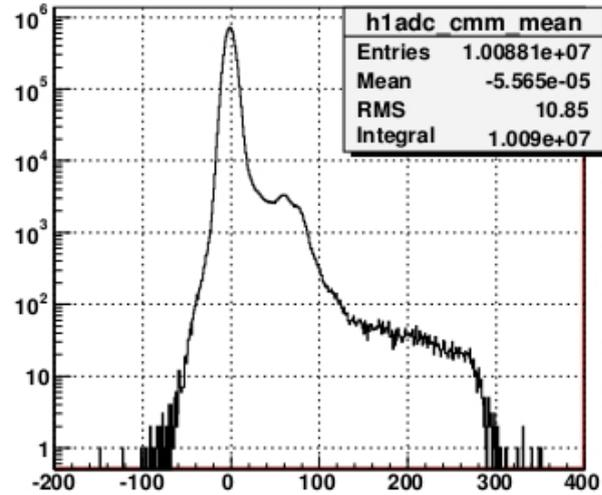
FIGURE 3.22: Histograms of Am-241 hit spectrum pixel distribution with noise peak and the right shoulder indicate the 59.5 keV peak (6<sup>th</sup> region of INTPIX3a).
