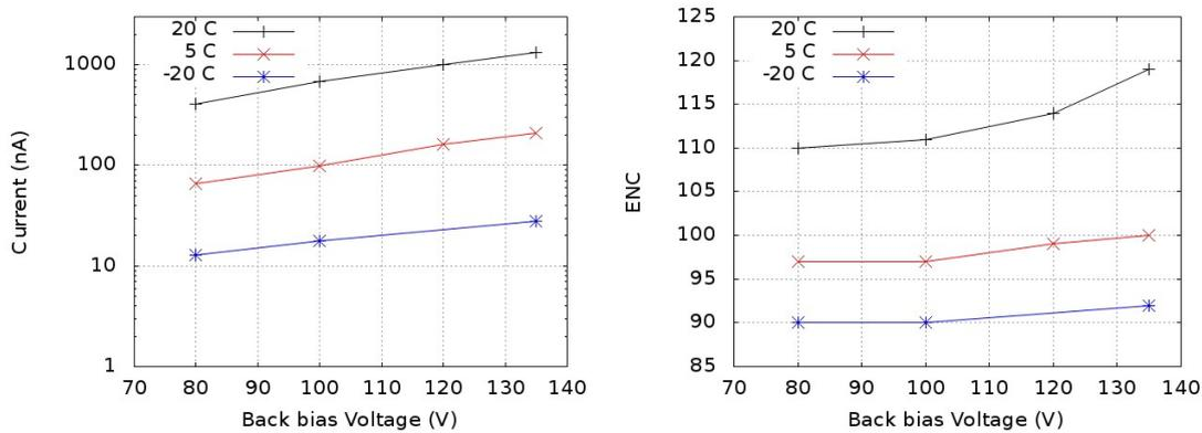
FIGURE 4.22: The CZ-n detector is measured to plot the leakage current (left) and ENC (right) as a function of detector bias voltage at three different temperatures.
