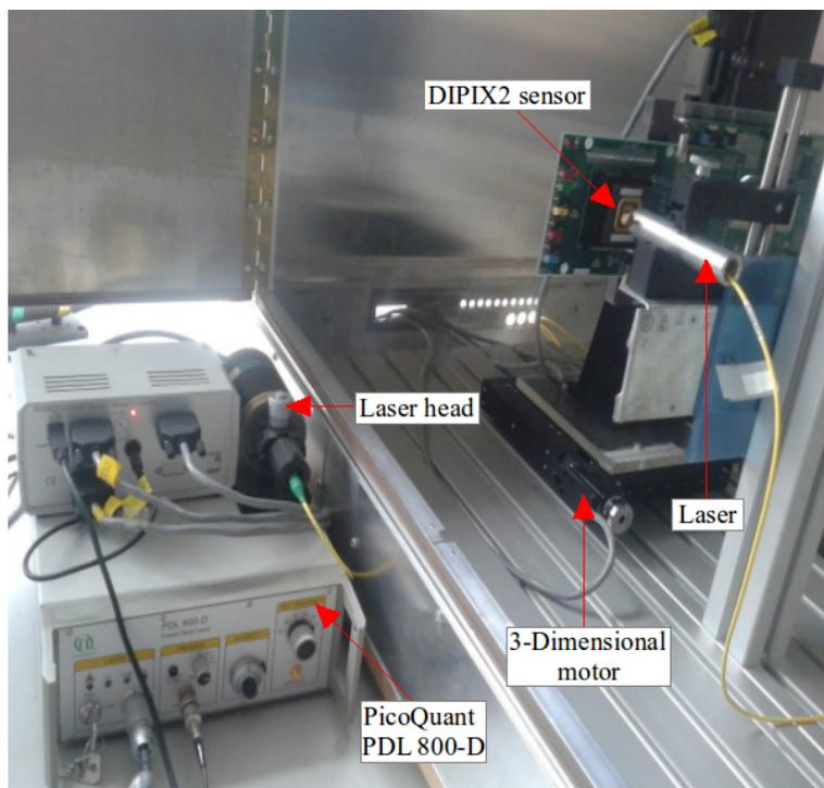
FIGURE 3.2: Laser set-up.
