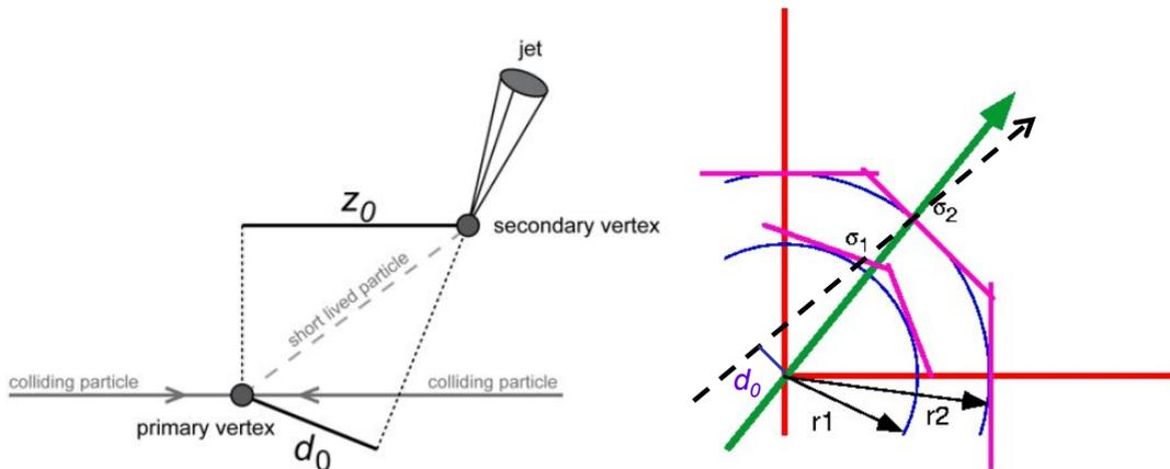
FIGURE 1.2: Illustration of impact parameters of short lived particle just a few  $\mu\text{m}$  (left) and simplified model of vertex detector to determine the impact parameter resolution (right). After [26, 27].
