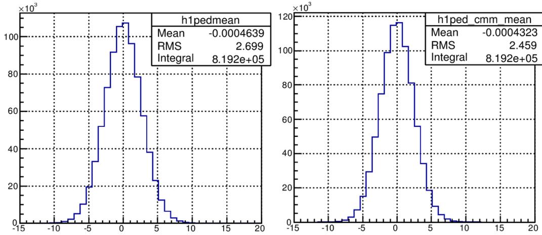
FIGURE 3.5: Histogram of 8<sup>th</sup> region of INTPIX3a without CM noise (left) and with CM noise (right).
