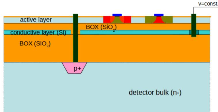
FIGURE 1.16: The concept of Double-SOI. After [84].
