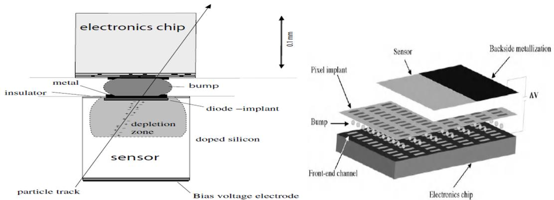
FIGURE 1.8: Schematic view of one pixel cell and a hybrid pixel detector. After [49].
