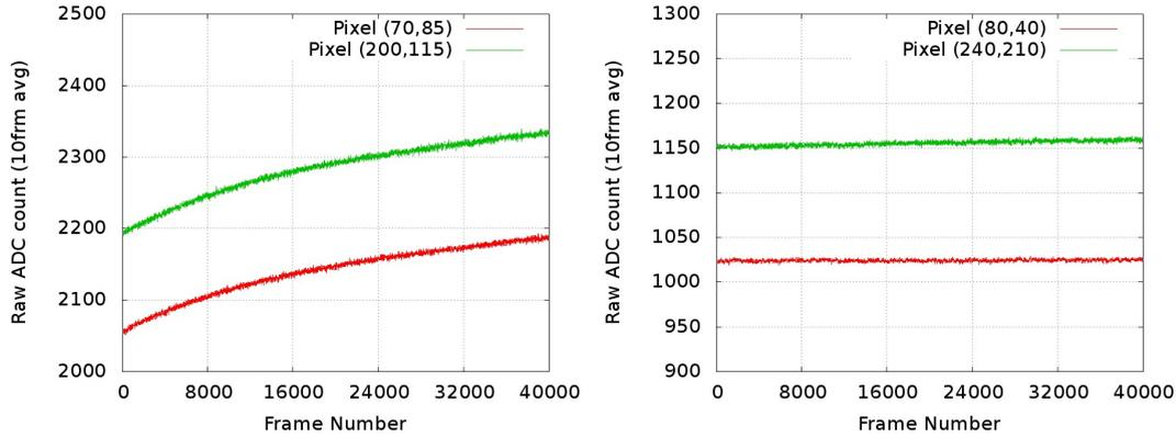
FIGURE 4.5: Long time stability test of DIPIX2 CZ-n (left) and FZ-n (right) detectors, pixel behaviour of two pixels, one from the 1<sup>st</sup> region and another from the 2<sup>nd</sup> region, is shown. It may be concluded that the DIPIX2 detector does not have the problem seen in INTPIX3 chip.
