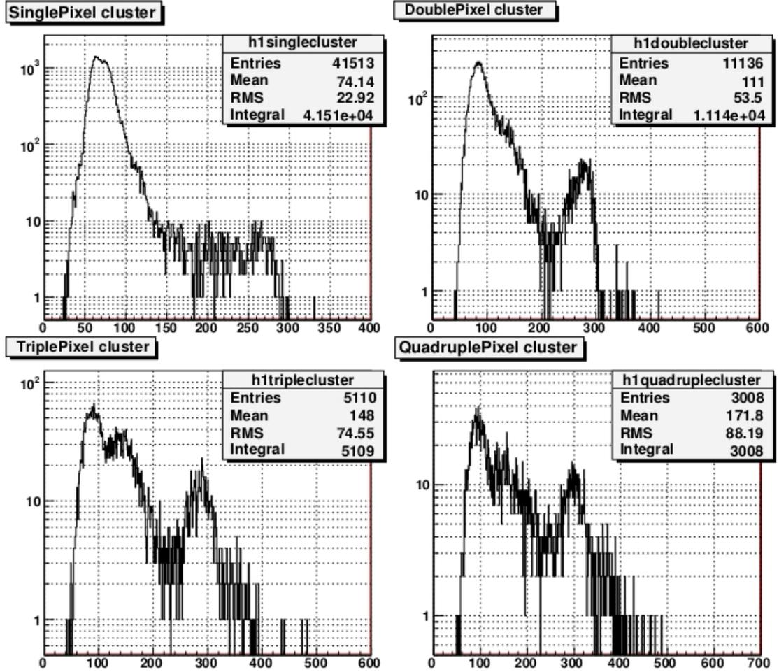
FIGURE 3.24: Histograms of single pixel (top left), double pixel (top right), triple pixel and quadruple pixel clusters are produced after exposing the detector to Am-241 source (6<sup>th</sup> region of INTPIX3a).
