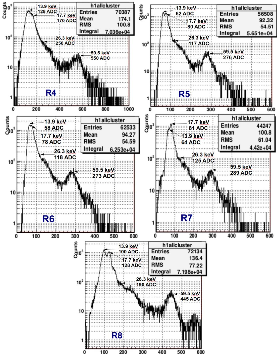
FIGURE 3.27: Histogram after merging all cluster of detector INTPIX3a.
