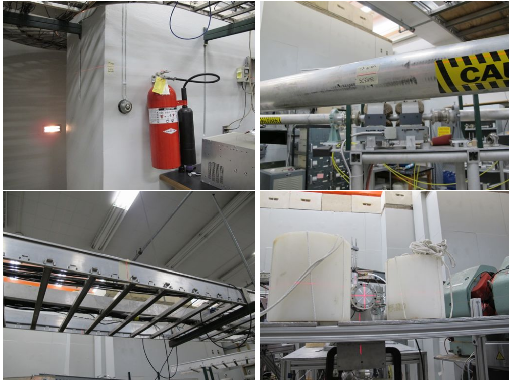
Figure 6.8: Aligning the laser. The laser was aligned with two pieces of tape at beam height on either side of the beam (Top left and top right) and a vertical line in front of (Bottom left) and behind the beam, as well as the target itself (Bottom right). The marks had been previously made by the SCENE collaboration.
