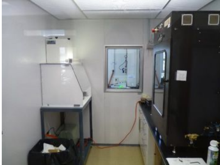
Figure 4.3: Dry room for crystal cutting and lapping/polishing at RMD. The room has a relative humidity level of 5%. The wire saw used for cutting is shown on the right while the dry box with HEPA filtration used for polishing is shown on the left. Image from RMD.
