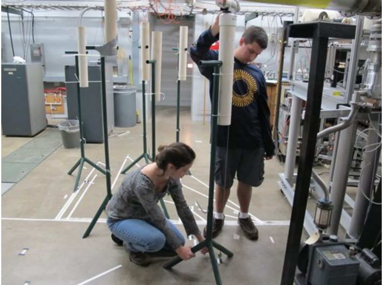
Figure 6.13: Centering the 5.1-cm detectors above the floor marks. In the picture is Shawn Westerdale and myself.
