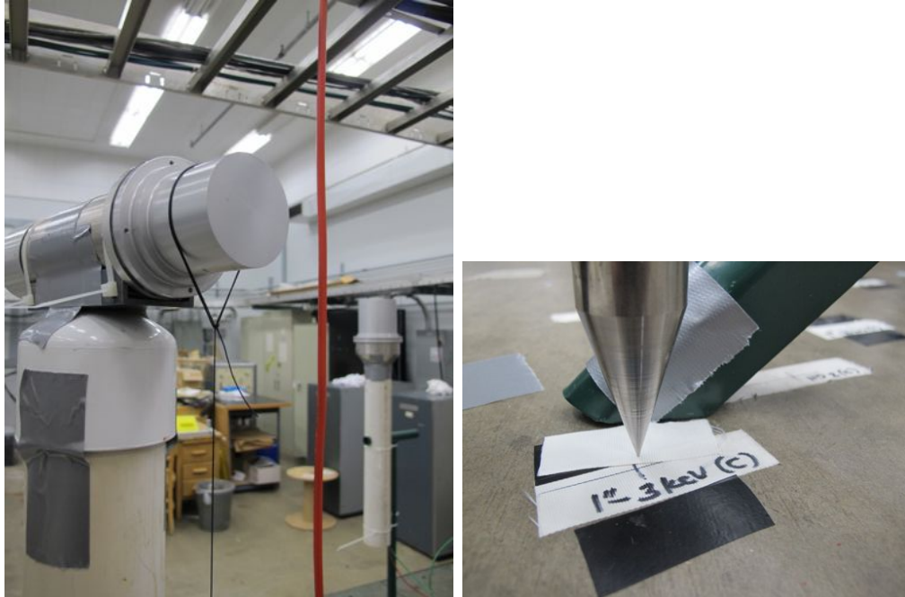
Figure 6.14: Marking the location of the 5.1-cm neutron detectors using a plumb-bob. The central location along the cylinder's z axis was measured and marked. A string with a plumb-bob on one end was tied around the detector loosely at this location, and the plumb-bob was allowed to hang from the center. The height was adjusted so the plumb bob was just above the floor, and the position of the detector was marked.
