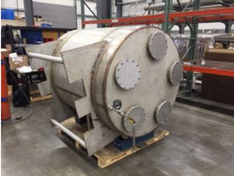
Figure 5.17: The SABRE portable veto-detector vessel, constructed at Allegheny Bradford Corporation. The vessel has been placed on a custom-made track so that it can be rotated freely.
