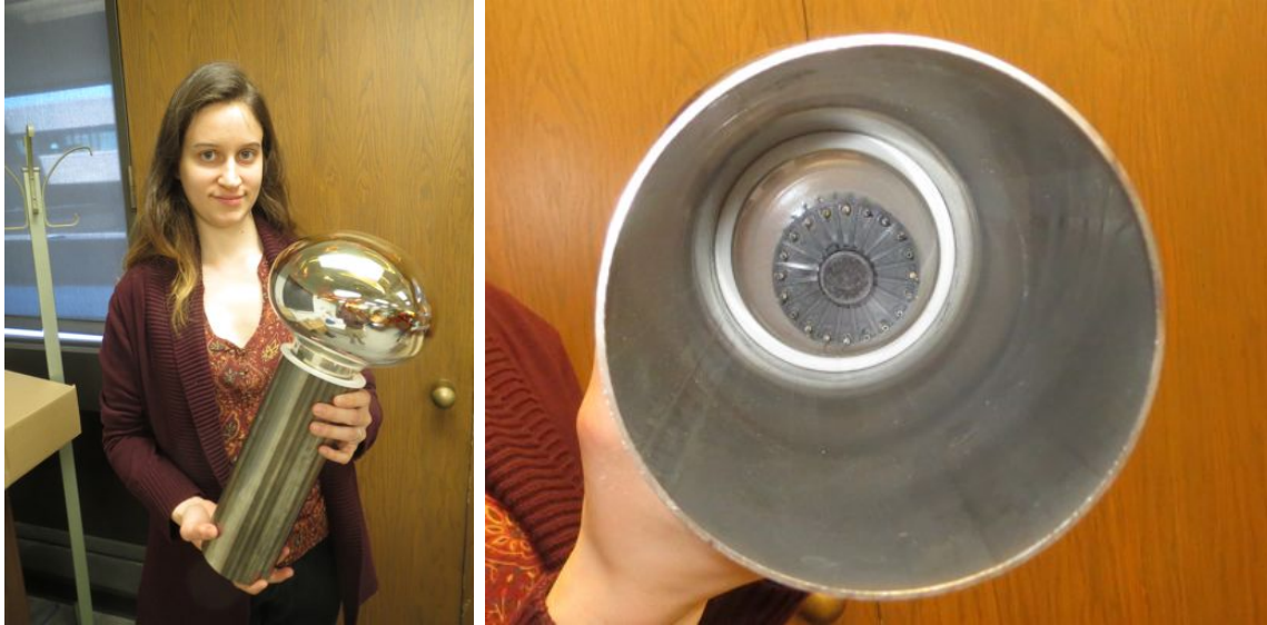
Figure 5.15: Test of the PMT grip design for the portable liquid scintillator vessel. A Teflon insert with o-ring grooves on both the PMT side and the can side creates a liquid-tight seal. This setup was tested with water for several weeks with no leaking observed.
