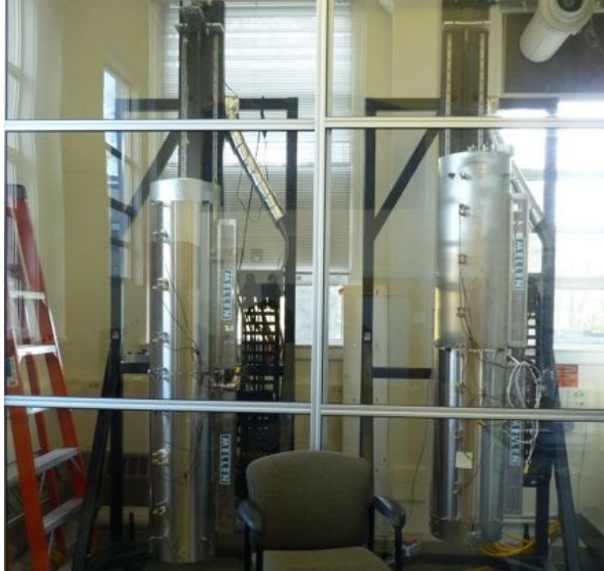
Figure 4.2: Furnaces for Vertical Bridgman growth, with maximum diameter of 13.3 cm. Image from RMD.
