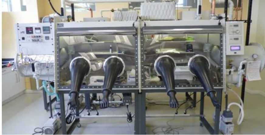
Figure 4.1: Glove-box used for crystal packaging at RMD. Parts coming into contact with the crystal are baked in the furnace on the left. The final polishing and packaging occur in this glove-box, which has a humidity level of around 1 ppm. A separate glove-box like this one is used for preparing crystals before growth. Image from RMD.
