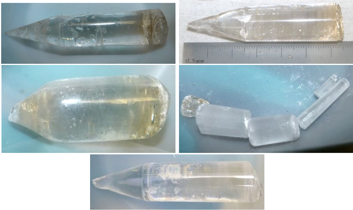
Figure 4.6: Crystals grown in the small crucible purity tests at RMD. G01 and G02 are in the top left and right, respectively, G03 and G04 in the middle left and right, respectively, and G05 at the bottom. Yellow appearance of some of the crystals is due to an optical effect of the camera. All of the crystals were colorless and transparent in the bulk. In the tails, there is some discoloration due to the segregation of impurities during crystal growth.
