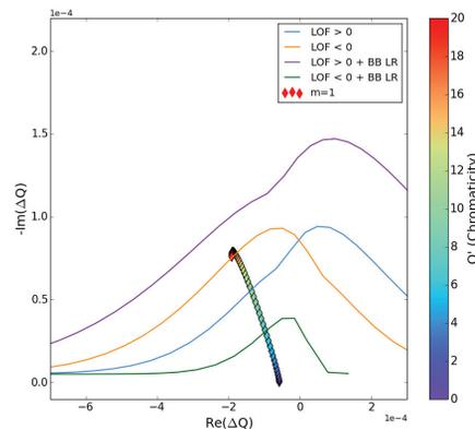
(b) Computed SDs with octupole magnets and LR beam-beam interactions. The head-tail coupled-bunch mode ( $m=1$ , Y-plane) is plotted as a function of the chromaticity value (color bar).
