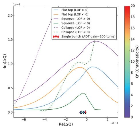
Figure 4: Stability diagrams at the minimum of stability during the collapse of the separation bumps for both octupole polarities. For comparison the SDs at flat top and at the end of the betatron squeeze are also plotted together with the most unstable single bunch modes computed for a transverse feedback gain of 200 turns (dots).
