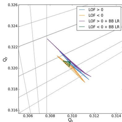
(a) Tune diagrams for negative and positive octupole polarity and LR beam-beam interactions.
