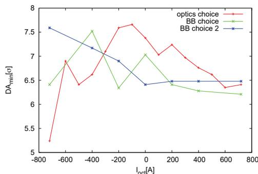
Figure 3: Dynamic aperture as a function of the octupole current and BB interactions ( $\beta^*=30$  cm) for various optics.
