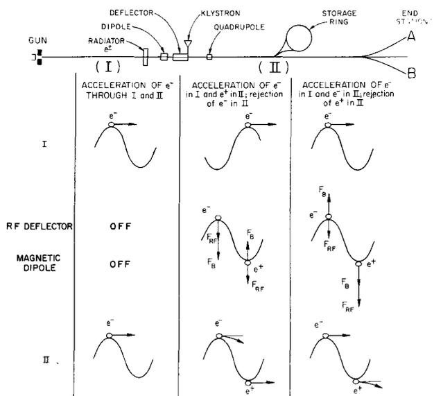
Fig. 5 - The three modes of operation of the electron-positron deflecting system.
