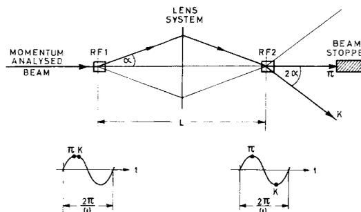
Fig. 1 - Principle of CERN r.f. separator.
