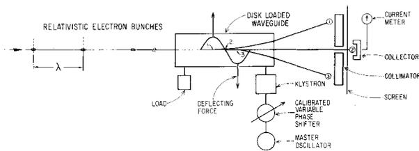
Fig. 4 - Deflector used as bunch-width analyzer.
