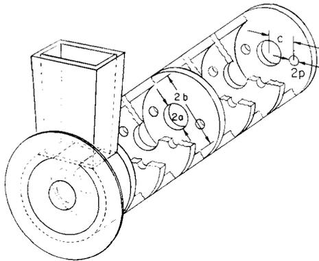
Fig. 1 - The « $TM_{11}$ -type» deflecting structure (LOLA).
