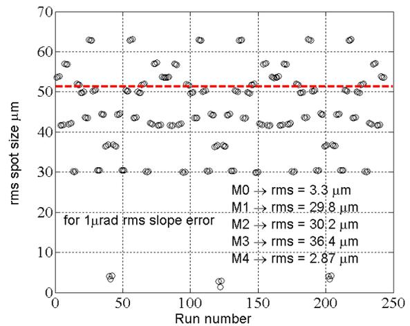
Figure 4: rms spot size vs run number for combinations of rms slope errors of -1, 0, 1  $\mu\text{rad}$  on the 5 mirrors; magnification of 1:1
