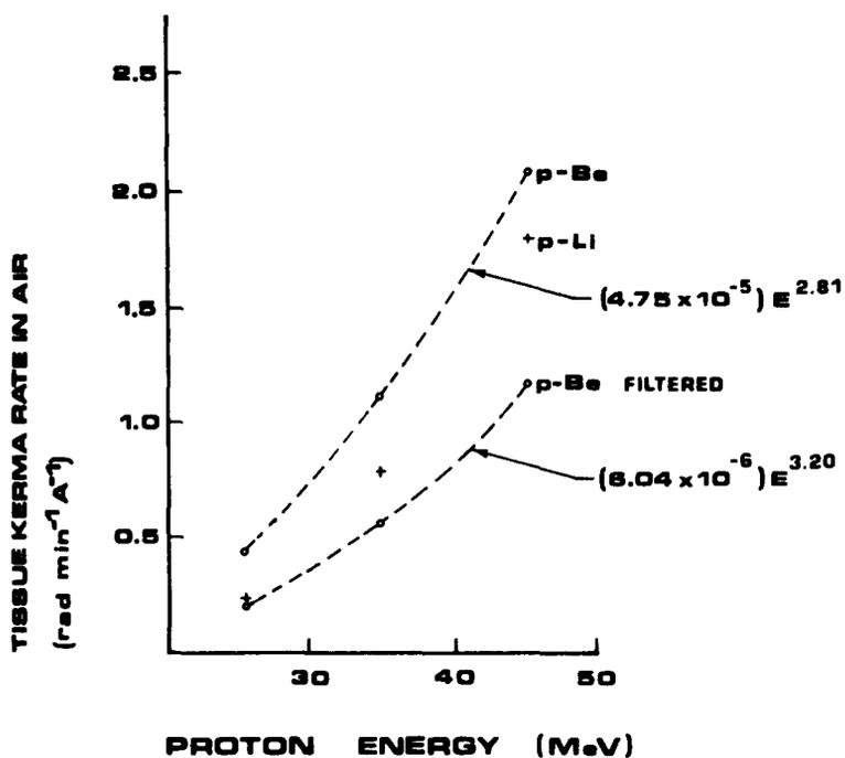
Fig.4.A. TISSUE KERMA RATE ( $n + \gamma$ ) IN AIR FOR  $10.7 \times 10.7$ cm NEUTRON BEAMS AT 125cm TSD.
