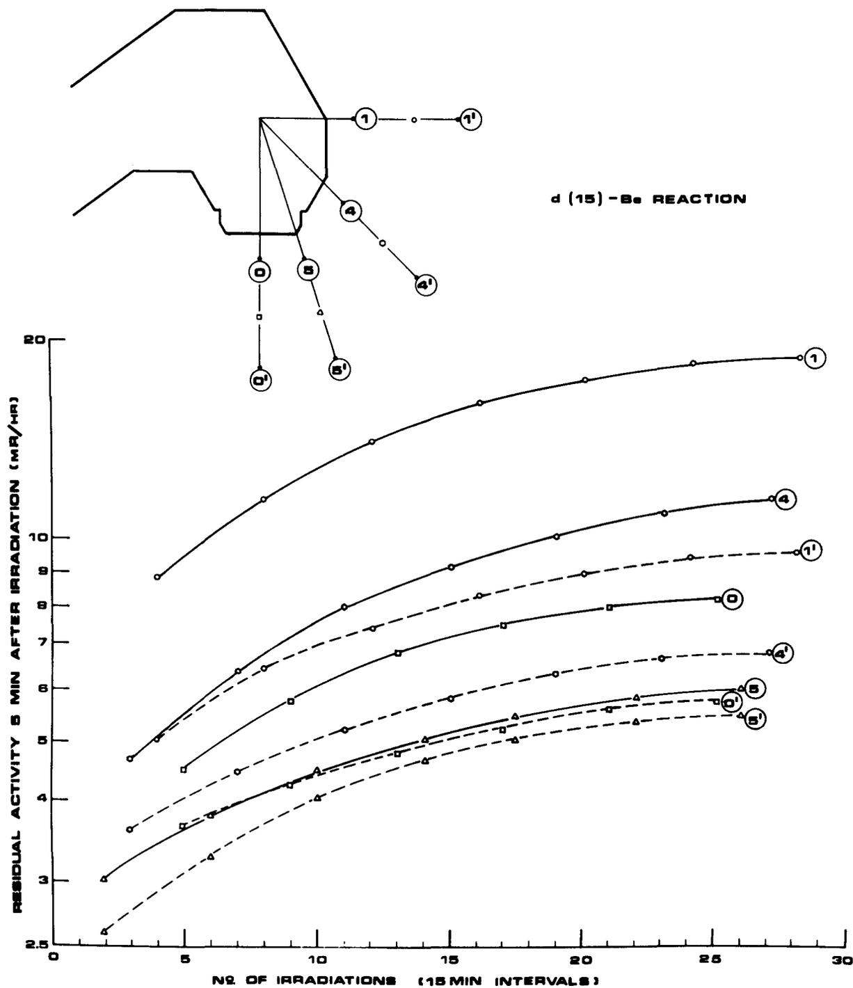
**Fig. 3 RESIDUAL ACTIVITY MEASURED 5 MIN AFTER IRRADIATION AND 20 CM FROM THE SURFACE AT DESIGNATED LOCATIONS. (SOLID LINE). BUILD UP WAS SIMULATED FOLLOWING A TREATMENT SCHEDULE OF 4 100 RAD FRACTIONS PER HOUR. BACKGROUND ACTIVITIES MEASURED 5 MIN AFTER IRRADIATION AND 1 M FROM THE SURFACE. (DASHED LINE).**
