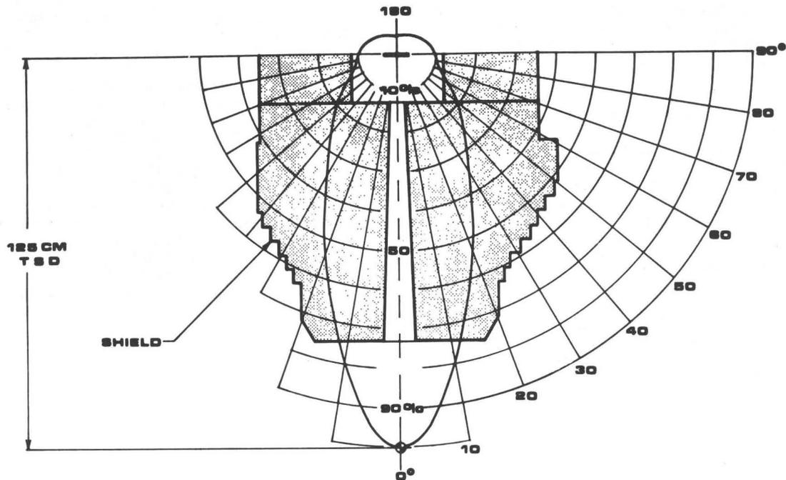
Fig.2.A. ANGULAR DISTRIBUTION OF FAST NEUTRONS FROM 15 MeV DEUTERONS SUPERIMPOSED ON SHIELD DESIGN FOR NEUTRONS FROM d,n REACTION WITH  $E_d=15$  MeV.
