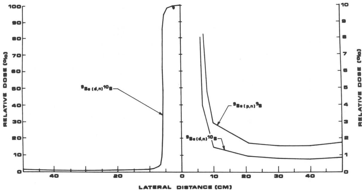
Fig.2.B. DOSE PROFILE MEASURED IN AIR, 10.7 X 10.7 CM FIELD AT 125 CM TSD.
