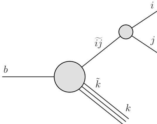
**Figure 2.3:** Schematic diagram of a splitting from a final-initial decay dipole that consists of the emitter  $\tilde{i}j$  and decayed spectator  $b$ . The recoil system prior to the splitting,  $\tilde{k}$ , is Lorentz transformed to absorb the splitting recoil momentum giving the recoil system  $k$ . The emitter following the splitting and the parton emitted in the splitting are  $i$  and  $j$  respectively.
