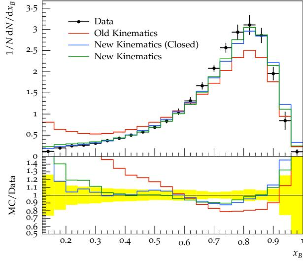
**Figure 2.1:** The scaled  $B$ -hadron energy distribution measured by SLD in electron-positron collisions at 91.2 GeV and predicted using the dipole shower. Predictions obtained using the previous implementation (Old Kinematics) of the splitting kinematics, the new implementation of the splitting kinematics with the ‘closed’ emission phase space (New Kinematics (Closed)) described in the text and the new implementation of the splitting kinematics (New Kinematics) are shown.
