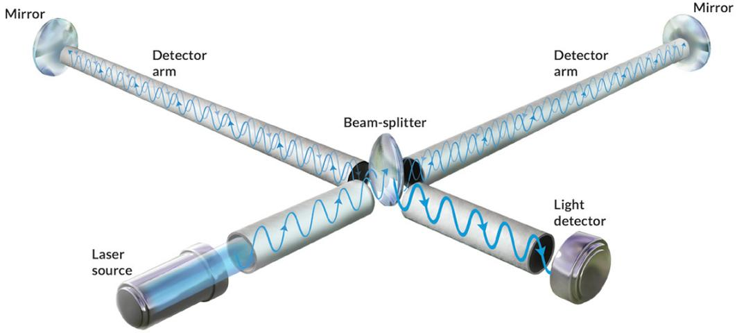
FIGURE 1.7: Schematic representation of a Michelson interferometer. A light beam is sent to a "beam splitter", where it is split in two beams: one which goes straight and another which is reflected by 90°. Both beams reach a mirror and are reflected back to the beam splitter that sums the signals and send them to a detector. Figure extracted from Ref. [165].
