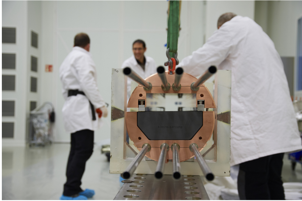
Figure 1.3. The SPS beam dump. In the picture, an absorbing graphite block is visible in dark grey. Image courtesy of Maximilien Brice.
