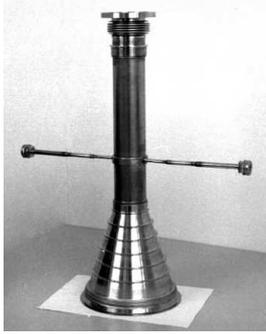
**Figure 2.5:** The central scattering chamber, made from 1.2 mm beryllium.
