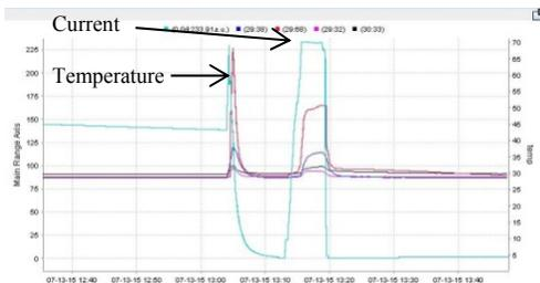
Figure 4: Temperature and current curve with bunch current over 10mA.
