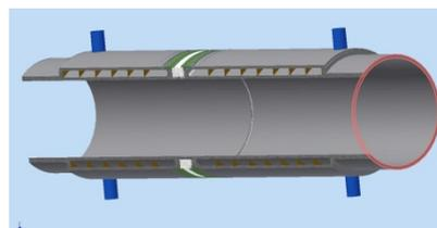
Figure 7: The interlayer of water cooling.
