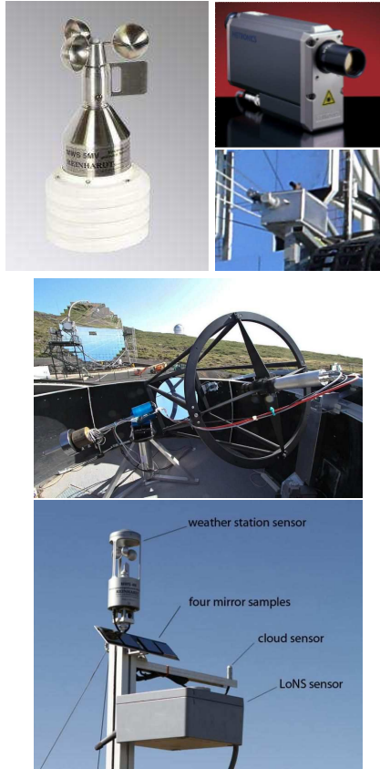
Fig. 1: Atmospheric monitoring instrumentation used at the MAGIC site. Top left: MWS 5MW. Top right: Radiation pyrometer and its installation attached to the MAGIC I reflector surface. Center: elastic LIDAR. Bottom: the Atmoscope unit.
