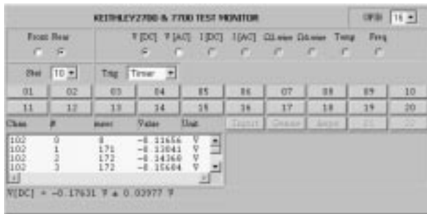
Fig. 4. The Keithley GPIB tool is used to configure and read channels from a model 2700 or 7700 multimeter.
