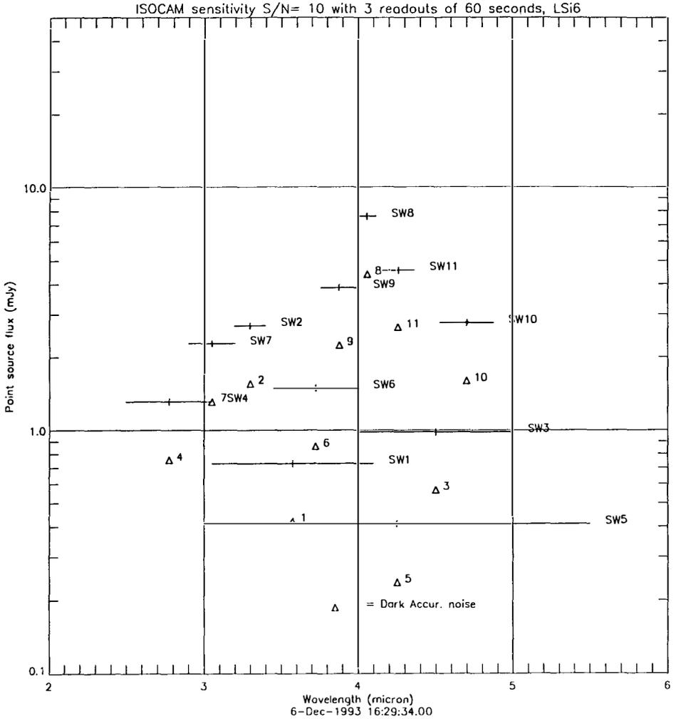
Figure 6. Point source flux giving a signal to noise ratio of 10, for all Short Wavelength filters, for 3 individual integrations of 60 minutes, and a 6" pixel field of view. At these wavelengths, the flat field noise due to the zodiacal background is negligible. The triangles represent the standard dark noise.
