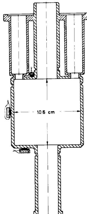
Fig. 1: Schematic drawing of S-band cavity with beam tubes. The cavity is constructed out of several niobium parts that have been electron beam welded together. The welds are shown as thinned walls in the drawing. Carbon resistors used to detect heat pulses are indicated schematically.
