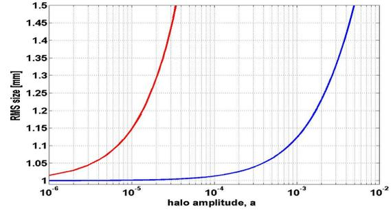
Figure 3: Dependence of the RMS size (blue line) and of the kurtosis (red line) on the halo amplitude for the profile of Fig. 2.
