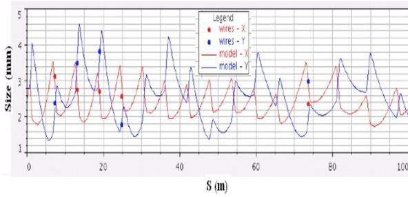
Figure 1: An example of beam size vs. distance along the SNS linac. Measured data are shown by dots.
