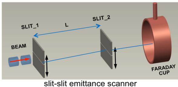
Figure 5: A schematic view of a slit-slit emittance scanner.
