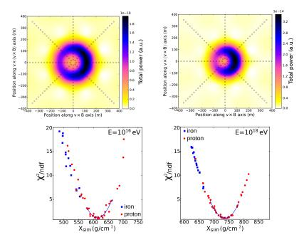
**Figure 5:** Top: Example simulated footprints of the radio signal in the shower plane for a proton-induced air shower, filtered to the frequency band of 50 - 350 MHz. Left: for a primary energy of  $E = 10^{16}$  eV, right: for a primary energy of  $E = 10^{18}$  eV. Reprinted from [9]. Bottom: Example  $\chi^2$  distributions for a proton-induced air shower with different primary energies. Left: for a primary energy of  $E = 10^{16}$  eV, right: for a primary energy of  $E = 10^{18}$  eV.
