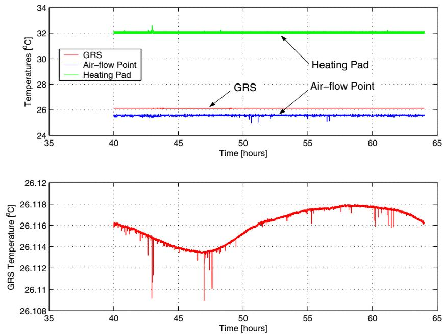
**Figure 4.** Time history of the GRS temperature: GRS, air-flow point, heating pad temperatures(top), GRS temperature (bottom)
