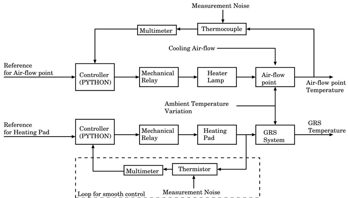
**Figure 2.** Control block diagram of the entire system
