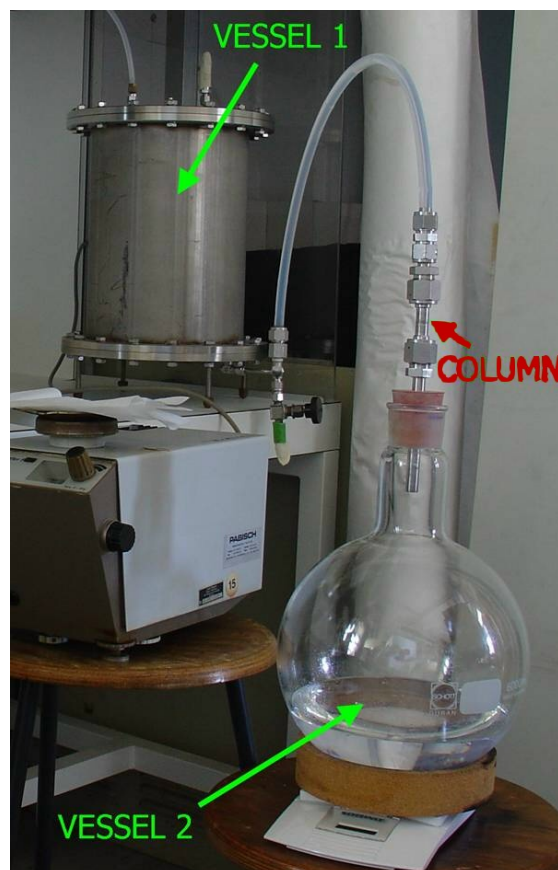
Picture 4.25: Set-up of the laboratory batch purification test
