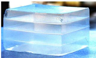
**Fig. 17** A stack of five Aerogel tiles, each one with different refraction index, to achieve focusing [26].
