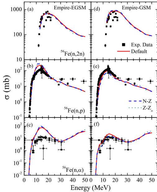
FIG. 1: Experimental and calculated cross sections of the reaction  $^{56}\text{Fe}(n, 2n)$ ,  $^{56}\text{Fe}(n, p)$  and  $^{56}\text{Fe}(n, \alpha)$ .
