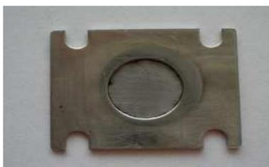
Figure 4.3: A front view of enrich chromium target deposited on gold backing
