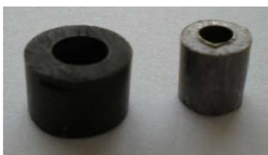
Figure 4.2: Graphite and Tantalum crucible used for keeping the target material inside plate to get a good quality target. By a good plate it means the inside surface of plate should be clean so that while pressing the plates any unwanted dust particle should not get inside the target. We have prepared  $\sim 12 \text{ mg/cm}^2$  gold foil for deposition of enrich target and  $\sim 4 \text{ mg/cm}^2$  for thickness measurement by alpha scattering method.
