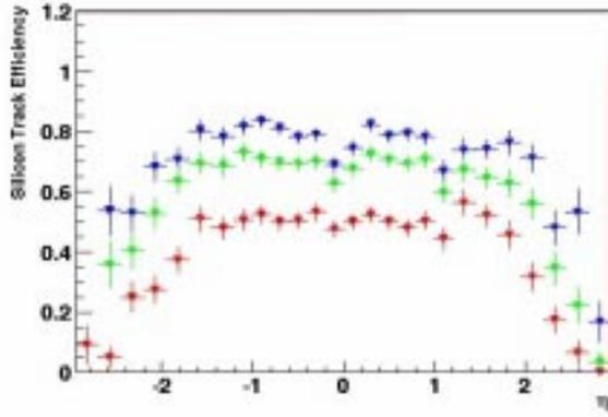
Fig. 1. Efficiency in data of the calorimeter seeded outside-in silicon tracking versus pseudorapidity for tracks with three(blue), four(green) and five(red) silicon hits.
