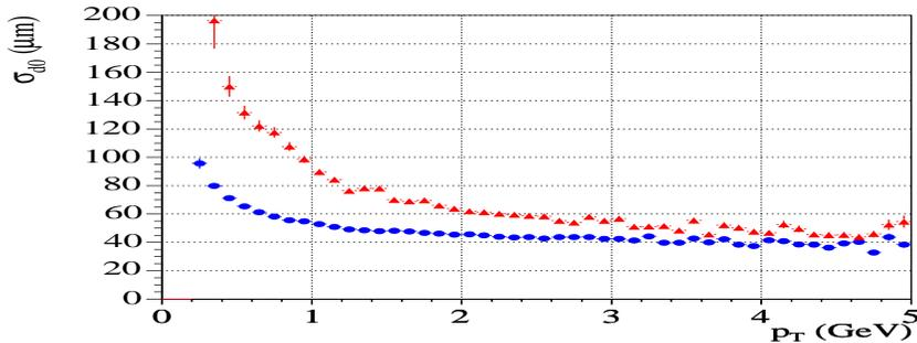
Fig. 2. Impact parameter resolution as function of  $p_T$  for silicon tracks passing through passive material. Red: Tracks without Layer 00 hits. Blue: Tracks with Layer 00 hits.
