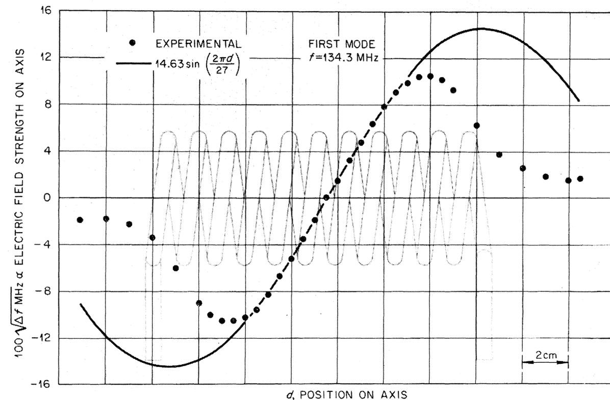
FIG. 2. Axial electric field in fundamental mode. The closed circles are the observed frequency shift as a function of position of the perturbing element along the axis of cavity. The solid line is a least mean square fit using the central points. The helical element is shown in the same scale for perspective.
