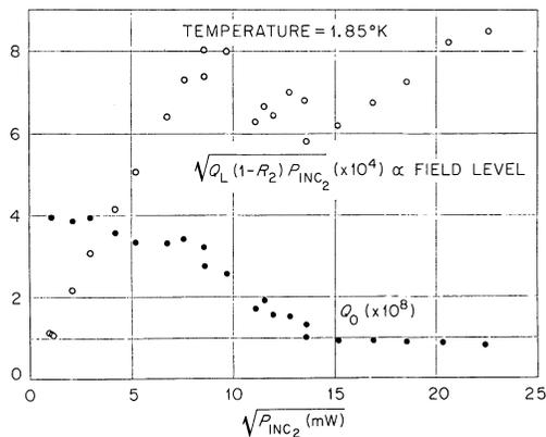
Cavity Filled with Liquid Helium.
