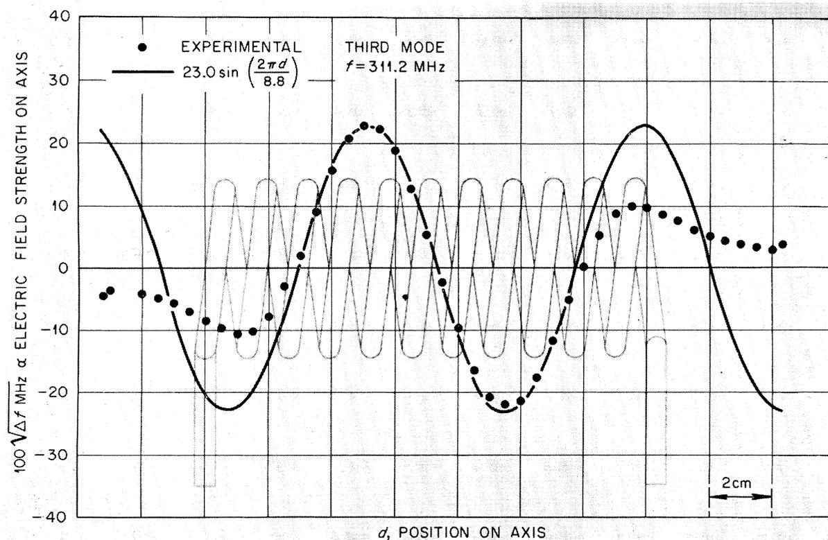
FIG. 4. Axial electric field in second harmonic mode. See Fig. 2.
