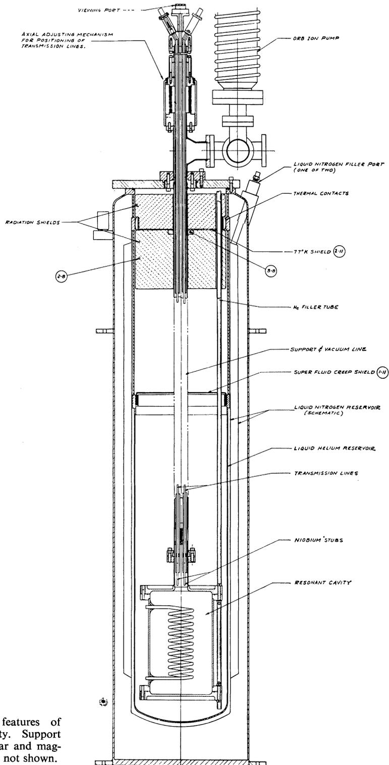
FIG. 1. General features of cryostat and cavity. Support structure for dewar and magnetic shielding are not shown.
