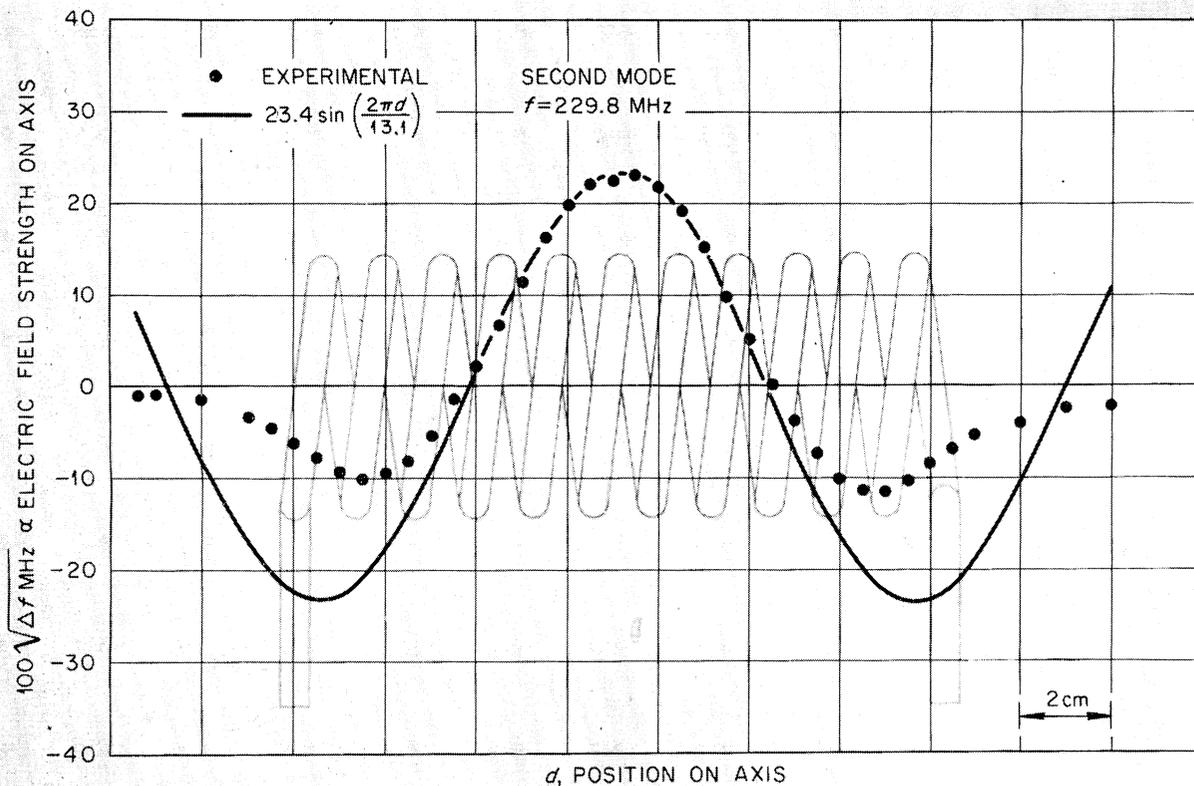
FIG. 3. Axial electric field in first harmonic mode. See Fig. 2.
