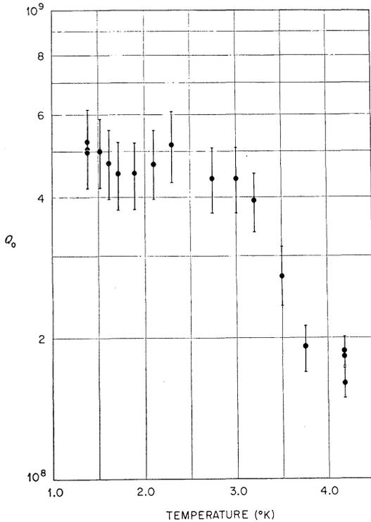
FIG. 6. Unloaded  $Q$ ,  $Q_0$ , measured as a function of temperature for transmission line position of '4 inch'.
