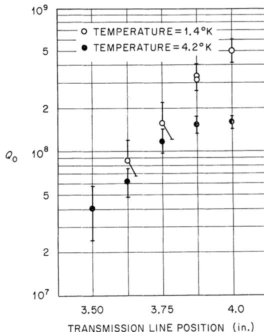
FIG. 5. Unloaded  $Q$ ,  $Q_0$ , as a function of transmission line position. The horizontal scale is an arbitrary measurement at the top of the dewar. Increasing values of this dimension correspond to withdrawal of the transmission lines.
