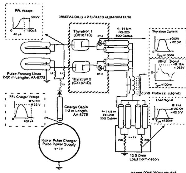
Fig.1 Simplified Schematic drawing of the kicker system
