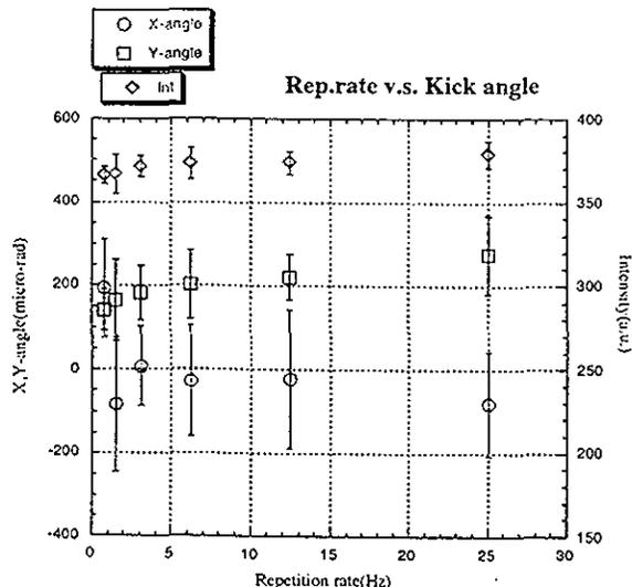
Fig. 7 Repetition rate characteristics
