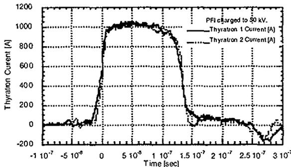
Fig.3 pulse shape of the thyatron currents
