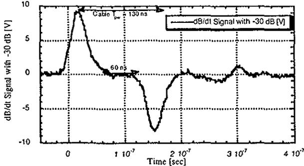
Fig.4 pulse shape of the dB/dt pick up
