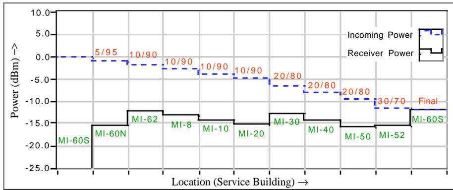
**FIGURE 2.** The passive splitting of a signal at each of the 10 service buildings. The top numbers indicate the splitter ratio while the top (dotted) line is the optical power in the incoming fiber to the service building. The lower (solid) line is the optical power to the receivers at each location with the name of the service building below the solid line. This calculation assumes a 1 dBm transmitter with a minimum receiver power requirement of -16 dBm.
