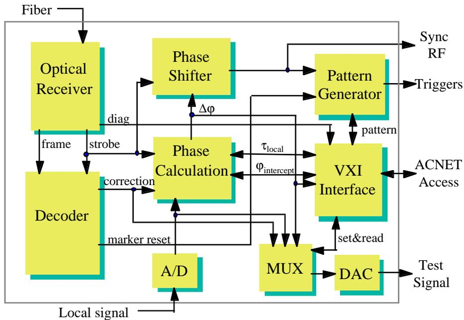
FIGURE 3. Diagram of the receiver.
