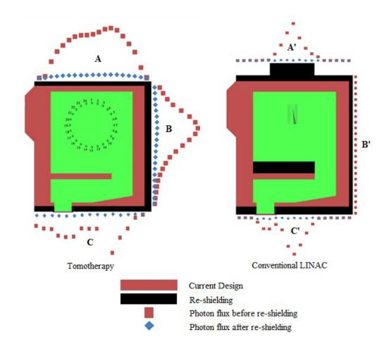
Figure 1. The photon flux distributions outside the Cobalt-60 room before and after re-shielding.
