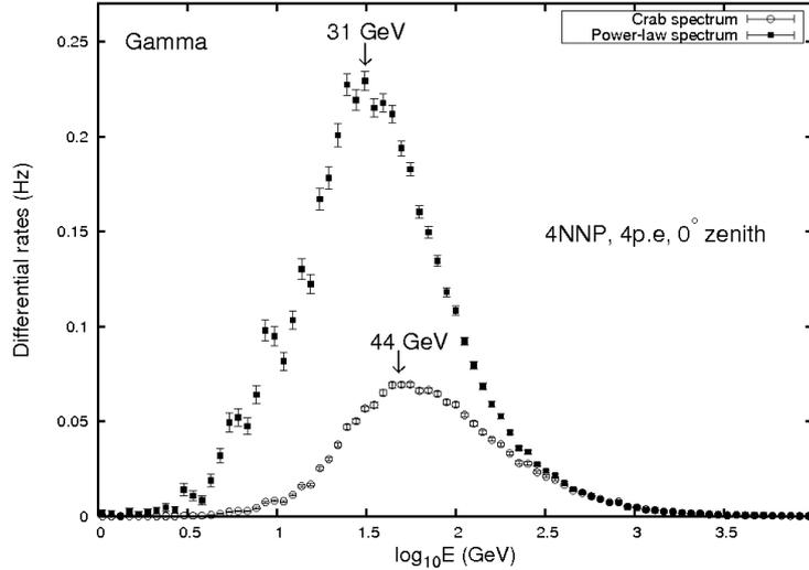
Figure 2: Gamma-ray differential rates for the two types of primary spectra calculated for the 4 nearest neighbour pixel, 4pe trigger con  $\sim (44 \pm 2) GeV$  and for the power law the threshold energy is  $\sim (31 \pm 2) GeV$ .
