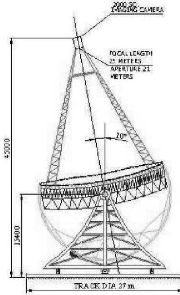
Figure 1: 21-m diameter MACE telescope
