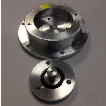
a. A custom-made vacuum feedthrough for the fiber optic cable, before assembly.
