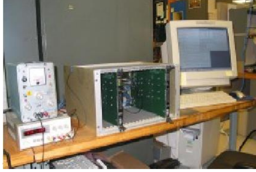
Figure A.8: The test stand pictured here was used to find the bit error rates from LVDS cables similar to those used in the platform and to check the track finding abilities using fake hit patterns sent at a rate similar to data taking conditions. After the upgrade, the test stand can also be used to test problematic boards.
