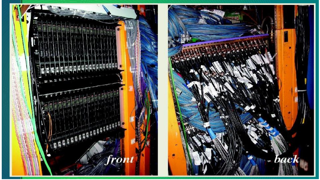
Figure A.9: The 40 DFEA2 boards are pictured here from the front (left) and back (right) view after being installed in the platform. The boards can be tested in the front end and easily removed since the wiring is all in the back of the crate.
