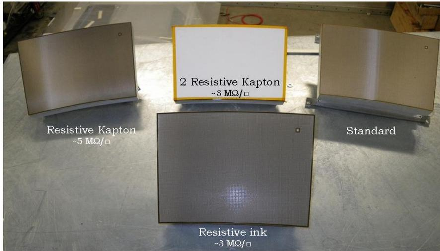
Figure 3-8. Five Micromegas modules with different anode materials.
