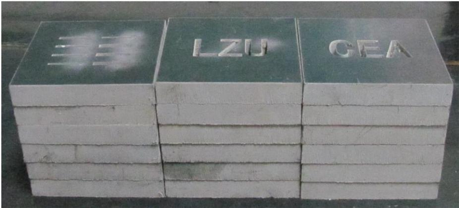
Figure 8-8. Polyethylene masks used for the neutron imaging.
