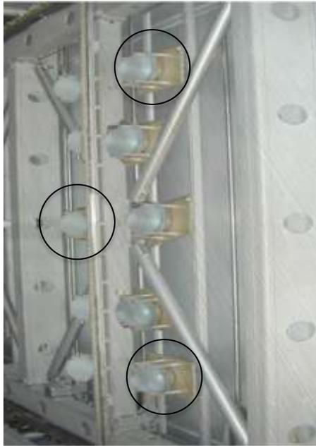
Figure 4.2: Photo-edited image that shows the possibility to install till 90 8''-PMTs on the existing T600 mechanical structure, by adding further PMTs in addition to the existing ones (circled).
