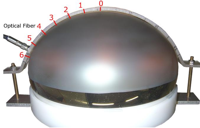
Figure 5.5: Support system used for photocathode uniformity measurements.
