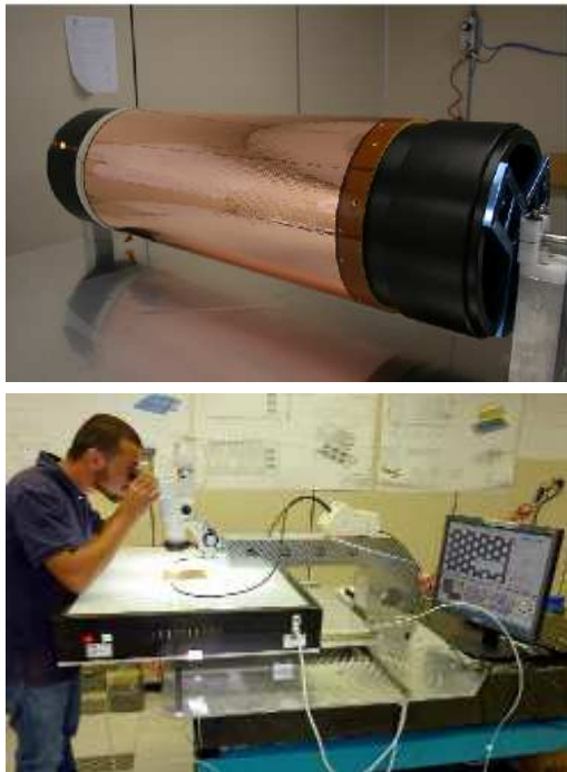
Figure 4. (Top) the aluminum moulds used for the construction of the cylindrical electrodes, (bottom) Visual Inspection tool.
