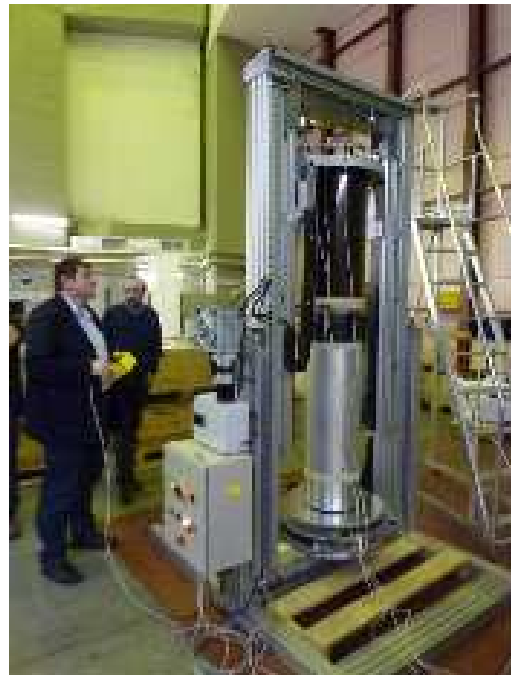
Figure 5. The assembly machine (VIS) used for the insertion of the electrodes one inside the other.
