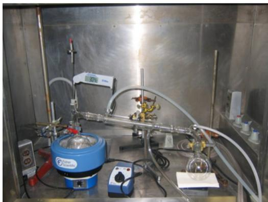
Figure 4.9: Vacuum distillation setup.
