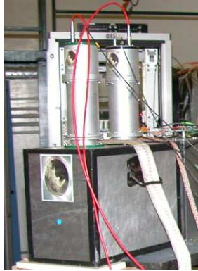
Figure 3.23: A photo of the Rino calorimeter. The bottom vessel contains 4 20 \times 20 \times 5 \text{ cm}^3 NaI blocks; the aluminum tubes contain two photomultipliers.
