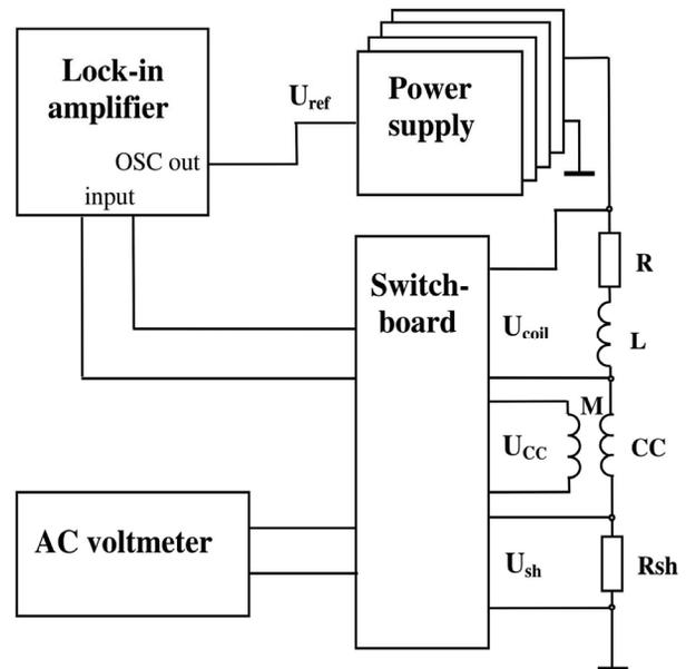
Figure 1: Electric scheme of apparatus for AC losses measurement in HTS coil.
