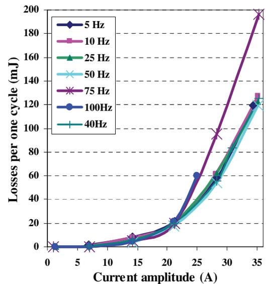
Figure 3: Dependence of AC losses on current in SuperOx coil without the iron core.
