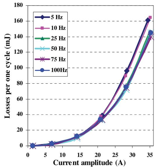
Figure 2: Dependence of AC losses on current in AMSC coil without the iron core.
