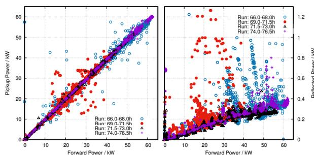
Figure 4: Pickup- (left graph) and reflected power (right graph) as function of the forward power.
