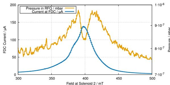
Figure 8: Measured effect of ion beam scrubbing.
