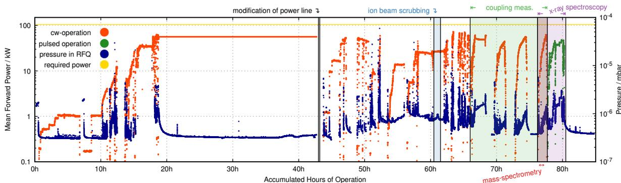
Figure 3: Accumulated operation hours of the RFQ since April 2016. The power for pulsed mode is the mean power at a duty cycle of 40%. After 43h hours of operation, the RF power line had to be modified. The periods of different measurements have coloured backgrounds.
