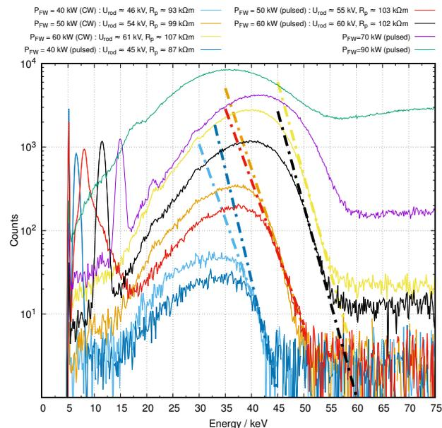
Figure 5: Spectra of x-ray spectroscopy for three RF power levels at CW-operation and six RF power levels in pulsed mode, resulting rod voltages and  $R_p$ -values.
