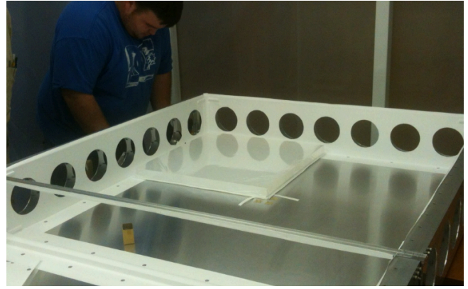
Figure 2: One Aerogel block being installed in the Super-TIGER C0 counter.
